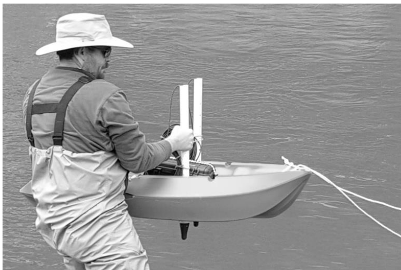
Figure 3. Data recording system and hydrophones mounted on a modified kayak being deployed on the Elwha River
