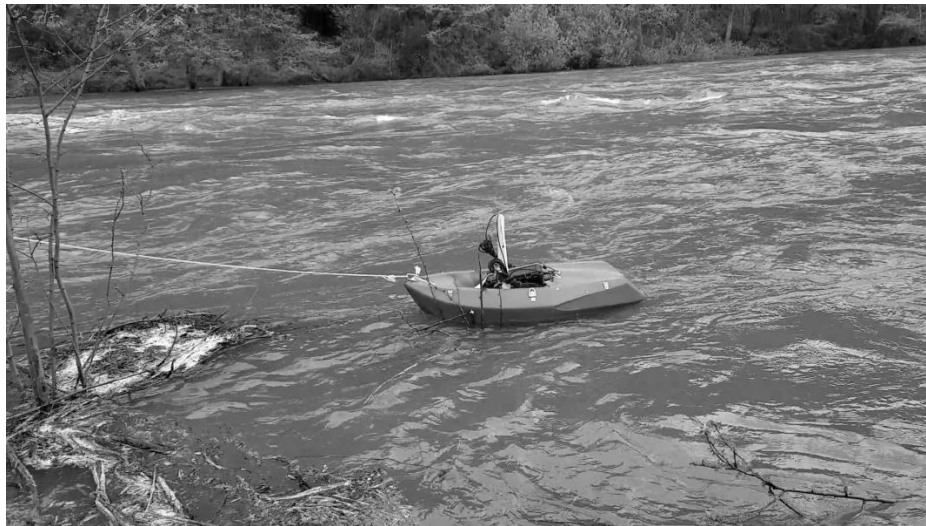
Figure 4. Hydrophone raft deployed on the Trinity River
