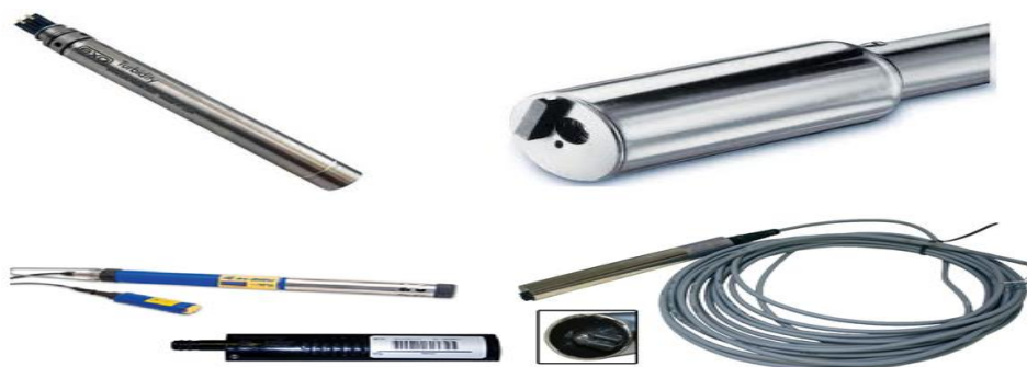
Figure 1. Tested turbidity sensors (right to left, and top to bottom); the EXO turbidity sensor, the HACH Solitax, the Aqua TROLL 600 turbidity sensor, and the ANALITE NEP-5000 by Observer
