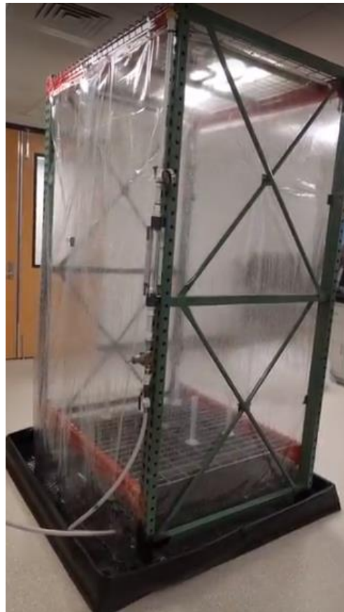
Figure 2. Rainfall simulator created for a laboratory setting.
