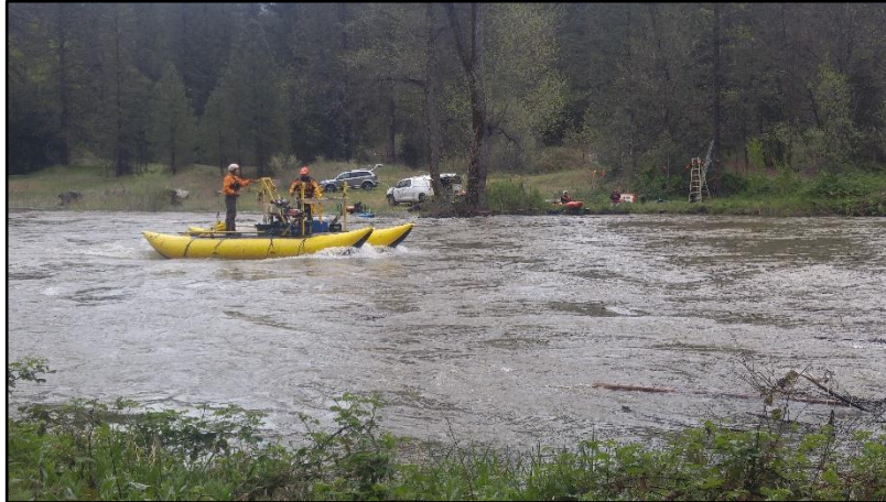
Figure 4. Trinity River near Douglas City, CA bedload sampling site. Discharge is approximately 13,000 cfs. The hydrophones were on both banks just upstream of the photo.
