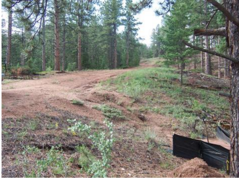
Figure 1. Unpaved road with drainage rill and a sediment fence to measure sediment production from a road segment on the Pike-San Isabel National Forest in central Colorado, USA.
