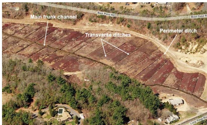
Figure 1. Cell 2 of the Eel River cranberry bog complex showing the central trunk channel, transverse ditches and perimeter ditches
