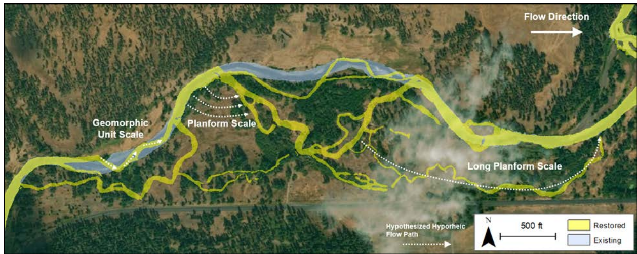
Figure 6. Existing (blue) and constructed (yellow) low flow planform of Bird Track Springs study area with hypothesized hyporheic flow paths.
