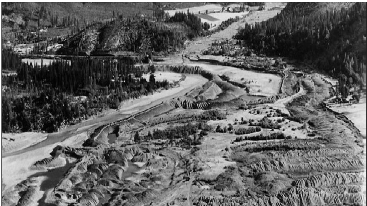
Figure 2. Trinity River dredger impacts. Note the removal of the riparian vegetation, the altered stratigraphy, and dredger tailing piles. The heavily placer mined Oregon Gulch flows into the upper center of the photo.
