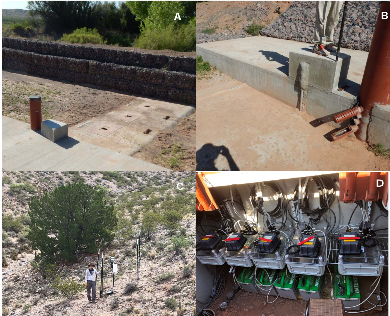
Figure 3. Overview of instrumentation. (A) Control section (view from right bank), with 3 Reid-type slot samplers and active acoustic surrogates upstream of slot openings. (B) stilling well for pressure transducer and two perforated arms housing ISCO pump sampler tubes and co-located turbidity sensors. (C) One of three up-basin rain gages to characterize rainfall-runoff relationship. (D) Control house with signal processors, data storage, and cellular data transmission. Control house also contains ISCO samplers (not shown).
