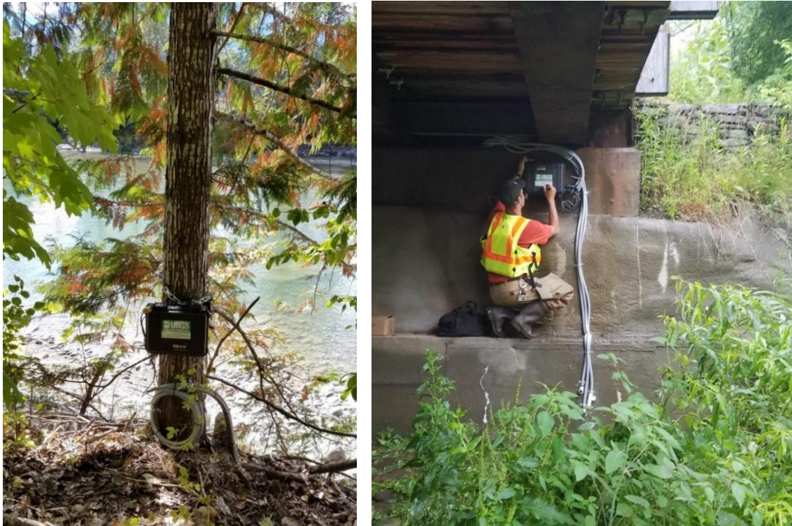
Figure 2. Examples of hydrophone installations: Sauk River, WA (left photo), Stony Clove Creek, NY (right photo)
