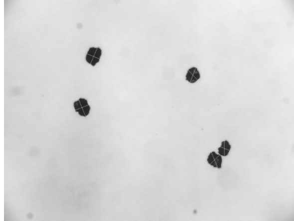
Figure 4. The perimeter and the A and B axis measured by the software are automatically highlighted. Two particles in the lower right were connected. The imaging software did a very good job measuring the particles separately.
