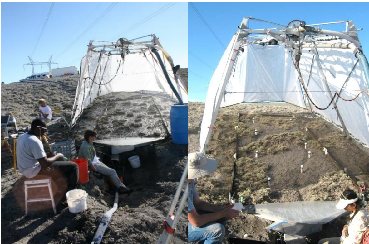
Figure 4. Walnut Gulch Rainfall Simulator operation at Dry X and DryX-II, Utah.
