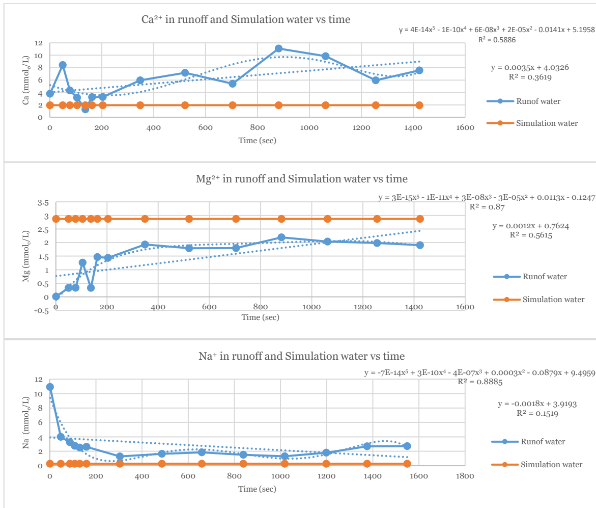
Figure 5. Concentration of Ca 2+ , Mg 2+ and Na + in the simulation water and runoff water for run 1 at Dry X with straight line and polynomial fits.
