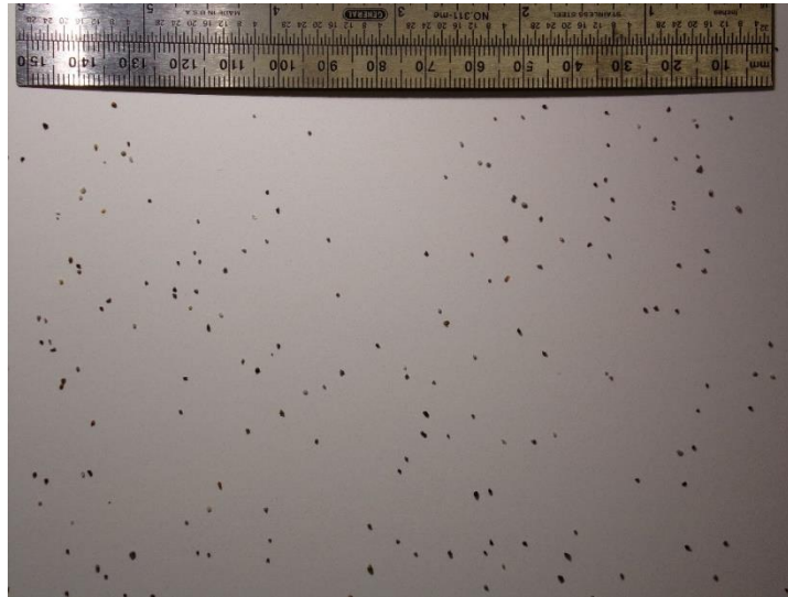
Figure 2. Sand size particles after being dispersed. Achieving a comprehensive particle dispersion can prevent misrepresentation of a Particle Size Distribution. Any particles overlapping may be interpreted by the software as a large single particle, biasing the distribution. (note: these particles were dispersed over a white surface and with a standard SLR camera just to show the pattern of particles after dispersion).
