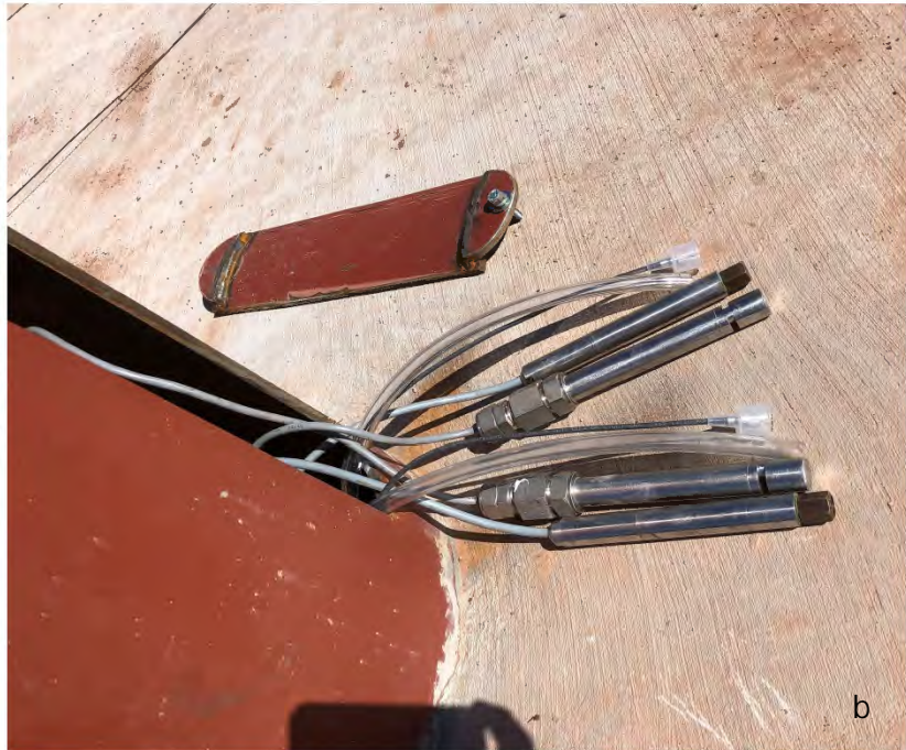
Figure 1: Stilling well with two perforated pipes attached; their vertical location is changeable. Suspended sediment monitoring includes a pair of the following instruments: intake for water sampler, sampler actuator, turbidity sensor and vented pressure transducer to actuate turbidity monitoring.
