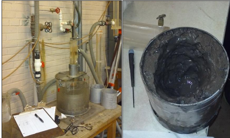
Figure 3. Laboratory Jet Erosion Tester (Left). Core 8 after testing (Right).
