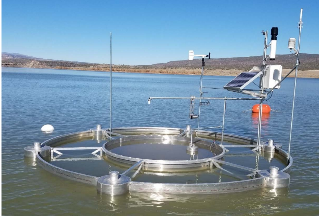
Figure 1. Collison Floating Evaporation Pan (CFEP) on Cochiti Lake, New Mexico (8-foot diameter evaporation pan and 16-foot diameter outer wave guard).
