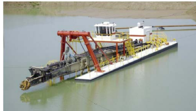
Figure 7b. Marlin Class Dredge Max Depth 96 ft. (std.), 200 ft. (custom) (DSC Dredge, LLC) vi
