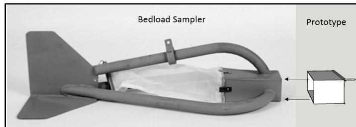
Figure 2. BL-84 bedload sampler and prototype of proposed attachment
