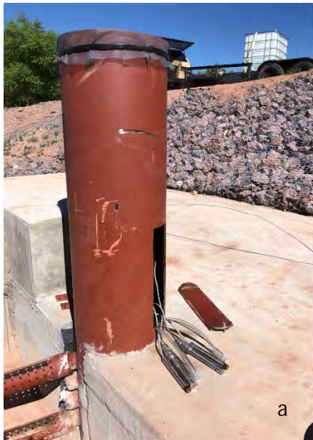
Figure 1: Stilling well with two perforated pipes attached; their vertical location is changeable. Suspended sediment monitoring includes a pair of the following instruments: intake for water sampler, sampler actuator, turbidity sensor and vented pressure transducer to actuate turbidity monitoring.
