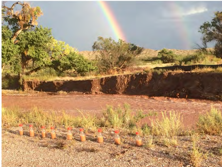
Figure 9. Suspended sediment samples (red-capped pint bottles, foreground) manually obtained during the June 10, 2017 flash flood. The color of the water indicates the relatively high SSC. View towards the left bank before deployment of the existing monitoring station.
