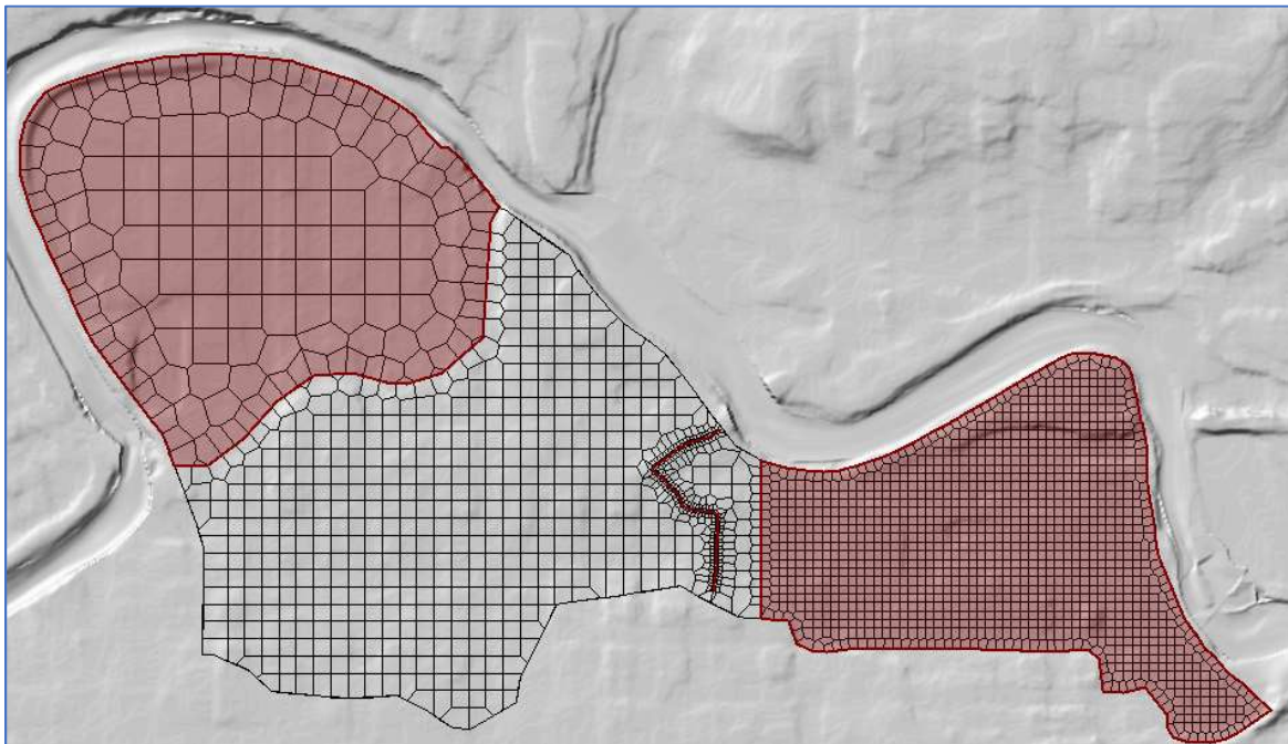
Figure 17. Example 2D model domain with an enforced breakline and refinement regions.
