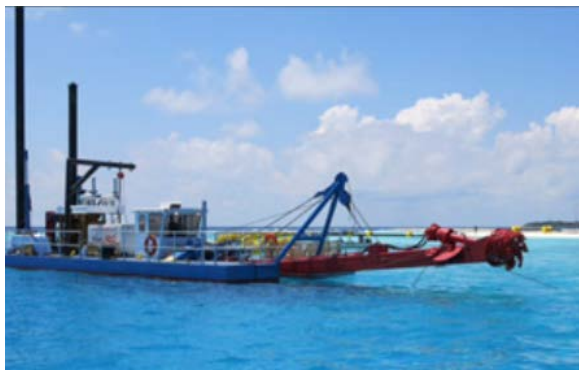
Figure 7a. Ellicott 670, Max Depth 42 ft. (Ellicott® Dredges, LLC) v
