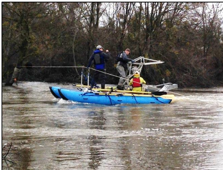
Figure 1. Tetra Tech engineers sampling bedload on the San Joaquin River in January 2017
