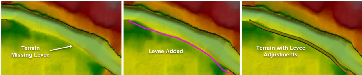
Figure 4. Process of adding high ground into a terrain.
