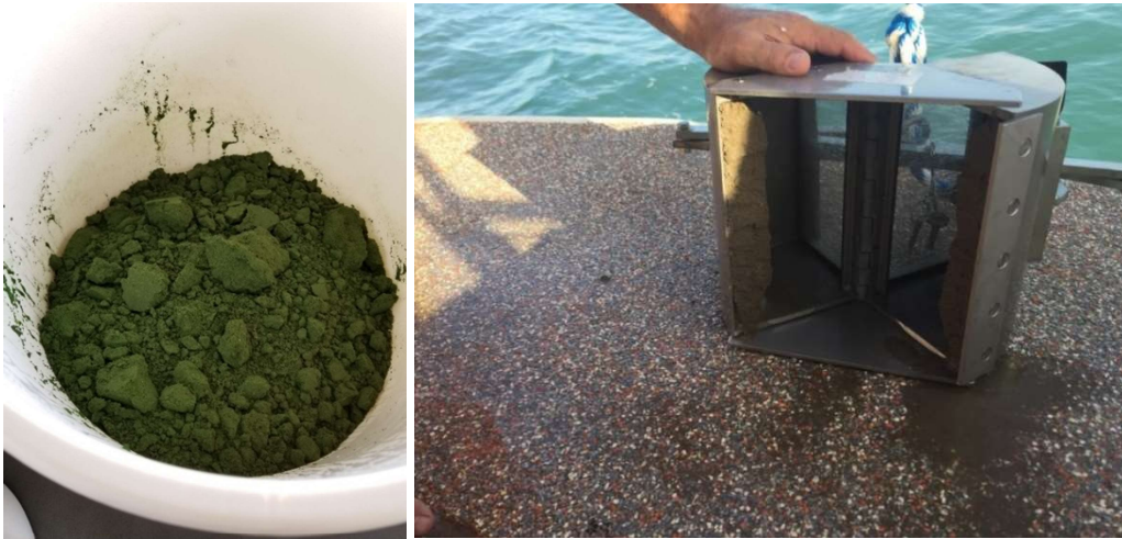
Figure 1. Tracer sand and sediment sampler used in the sediment tracking study.
