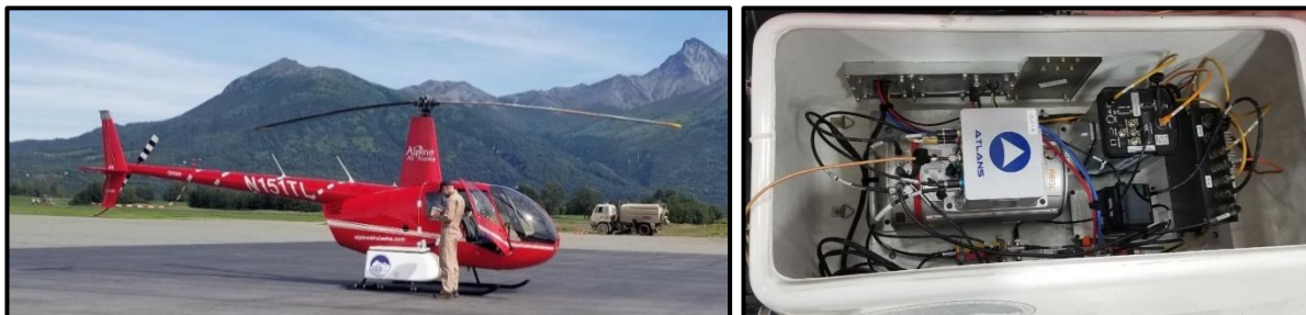
Figure 1. HeliPod mounted on R44 Raven II Helicopter and top view of 2018 HeliPod instrumentation payload
