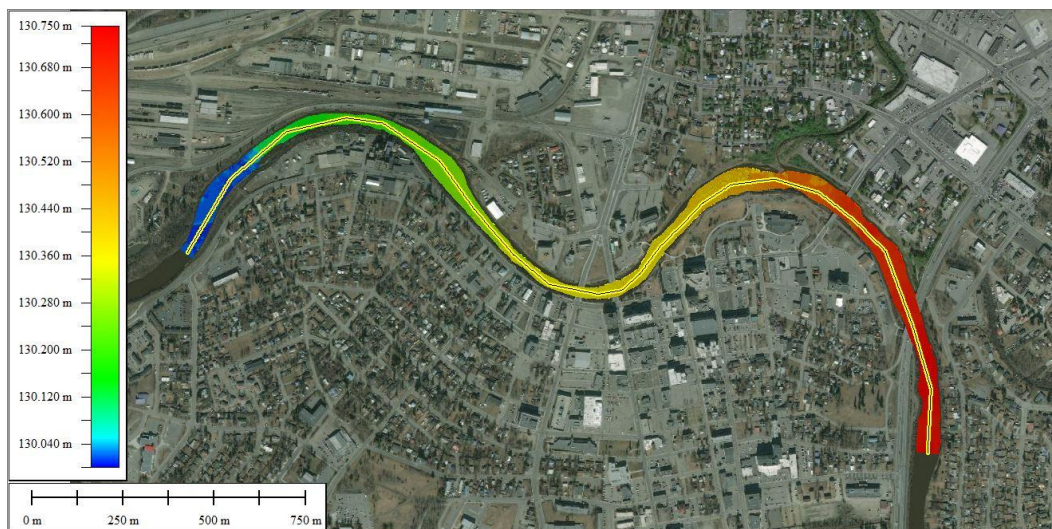
Figure 3b. Map of interpolated lidar water-surface elevation and profile (yellow) for the Chena River in 2017
