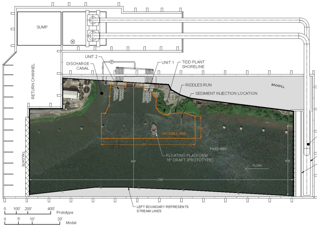
Figure 5. Plan view of the 1:24 scale physical model
