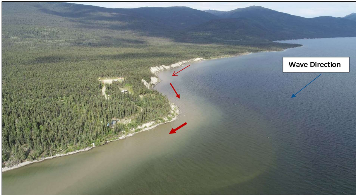
Figure 4. Northern side of Outlet Channel entrance; red arrows indicate longshore sediment transport (NHC 2018)
