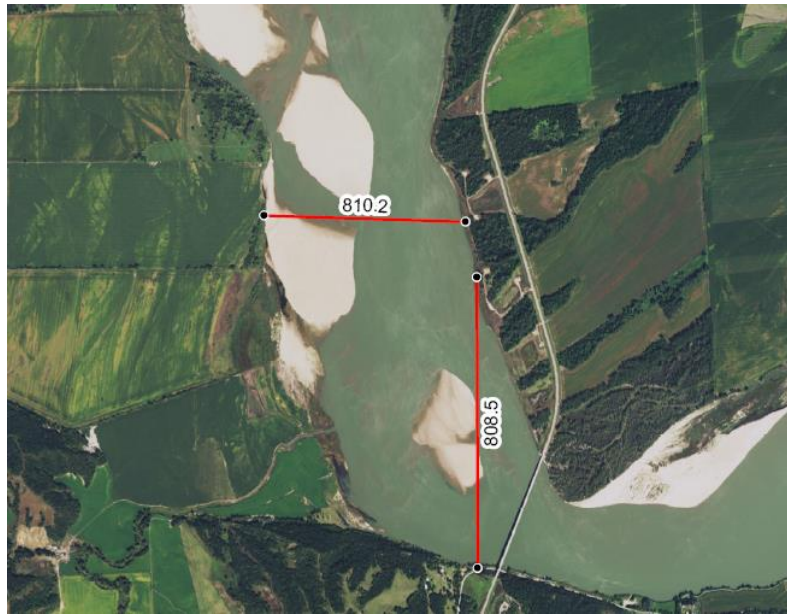
Figure 1. An example of the potential for erroneous bank change calculations due to channel migration. Range line labels refer to 1941 river mile markers. The channel has migrated such that the survey range line in the lower-right corner becomes essentially parallel to the channel. Erosion of the river-left bank occurring below range line 810.2 would be erroneously captured in repeated surveys of range line 808.5.
