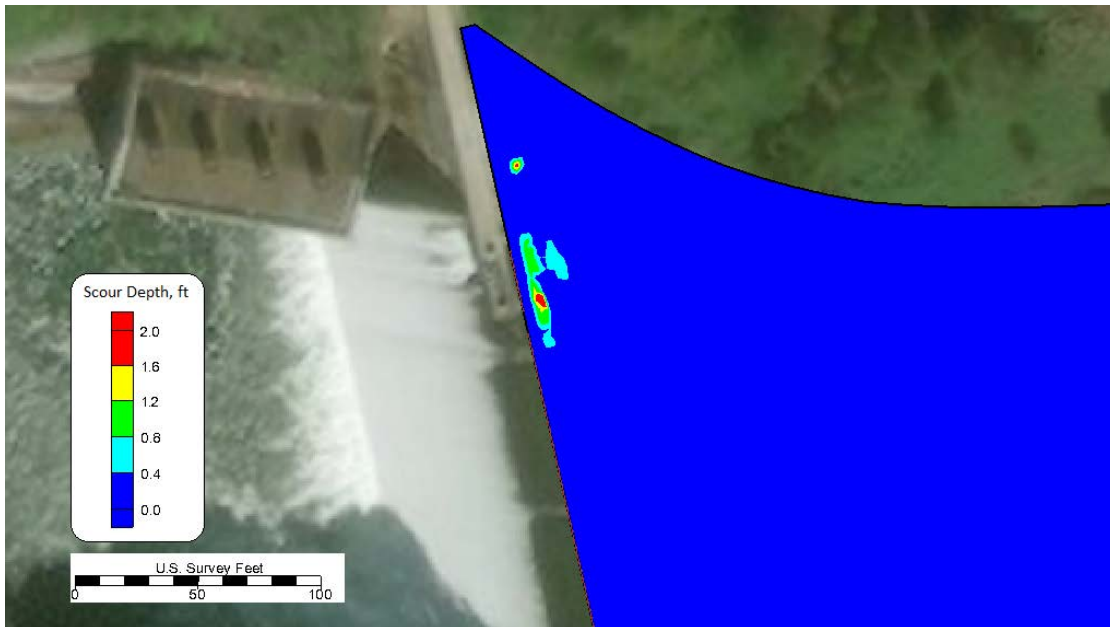
Figure 17. Scour depths near the gate
