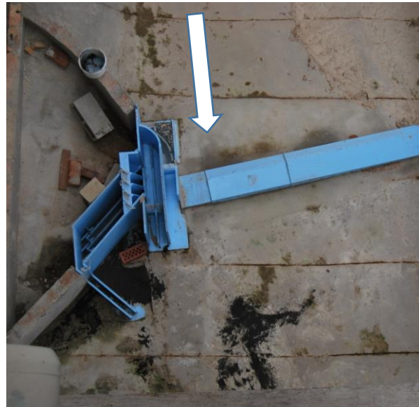
Figure 8. Plan layout of the undistorted model of the abstraction works and weir
