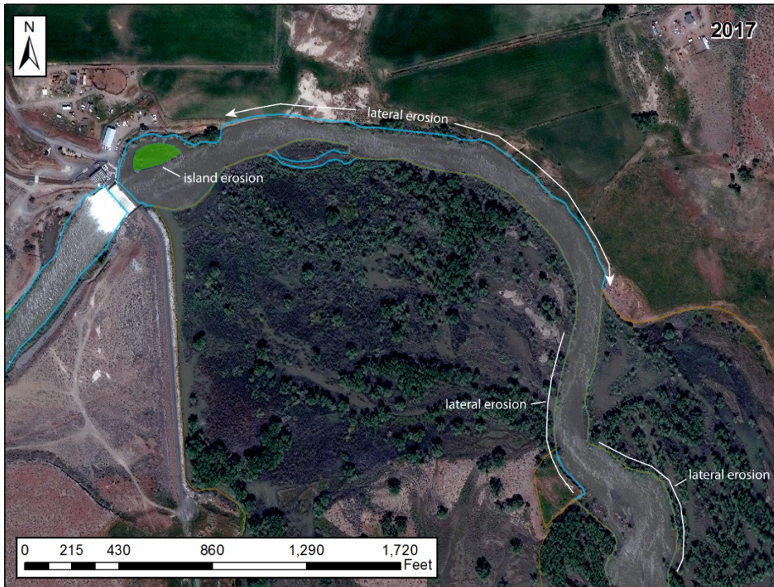
Figure 11. 2017 aerial photograph showing channel changes upstream of Marble Bluff Dam as a result of the 2017 flood.
