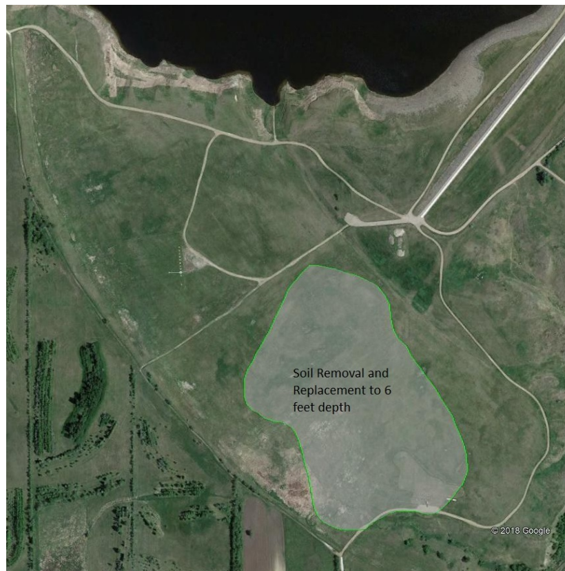
Figure 2. Areal Extent of Surficial Sands Removed from Spillway During Construction.
