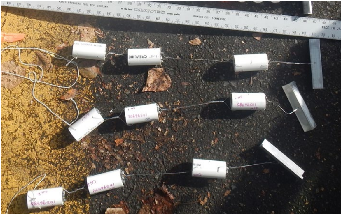
Figure 2. Three scour chains equipped with accelerometers prior to installation
