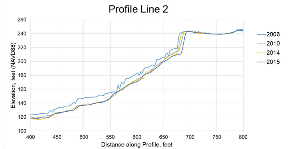
Figure 11. Profile through scour hole (Hickman Hardpoint at Distance 695).
