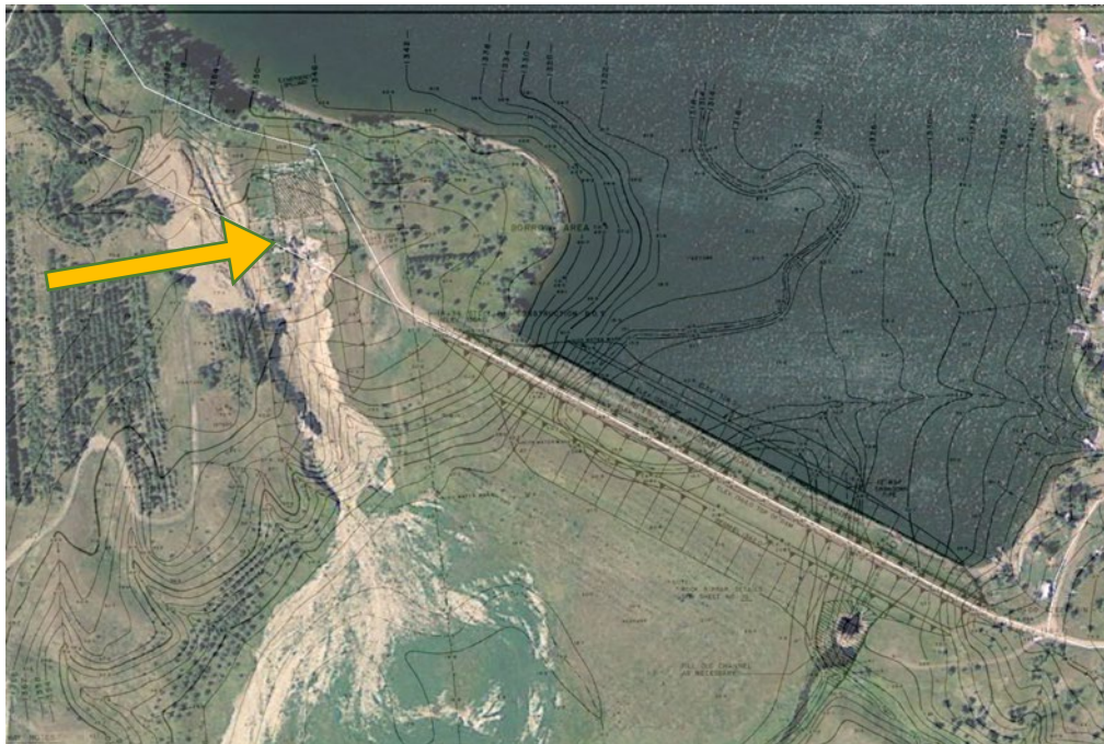
Figure 3. Post-flood aerial imagery of Cottonwood Creek Dam. Orange arrow calls out upper extent of head cut, approximately 40 feet from the crest.
