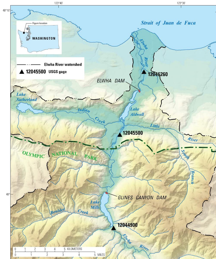
Figure 1. Elwha River basin prior to the start of dam removals in September 2011, showing the locations of the former Elwha Dam which formed Lake Aldwell and the former Glines Canyon Dam which formed Lake Mills.
