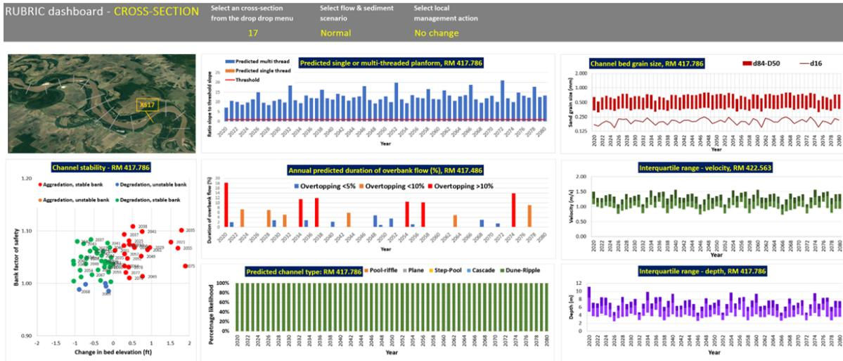
**Figure 4.** Example dashboard for channel evolution through time (2020–2080) at an individual cross-section. Simulation for cross-section 17 on the lower Mississippi River assuming a sequence of future flows very similar to those of the recent past (see text for details).
