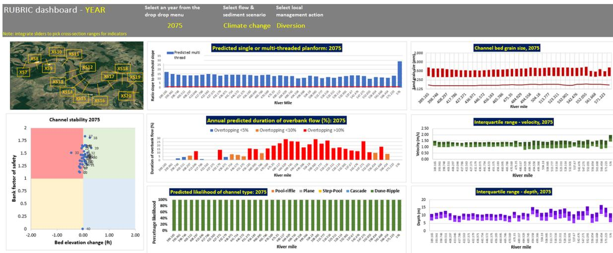
**Figure 5.** Example dashboard for channel evolution along a reach for an individual year. Simulation of change along the lower Mississippi River by 2075 (part of a simulation 2020–2080) assuming a flow diversion operates during flows >400,000 cfs part way along the reach, and that flow conditions are significantly wetter than in the recent past (see text for details).
