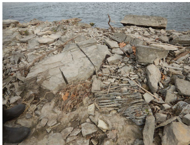
Figure 4. Rock weathering and disintegration in a structure on the Republican River, KS.
