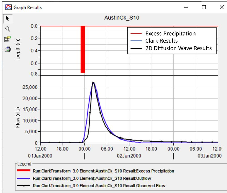
Figure 3. Example of Calibrating Clark Unit Hydrograph Parameters to Match 2D Diffusion Wave Results for 3 in/hr Excess Precipitation
