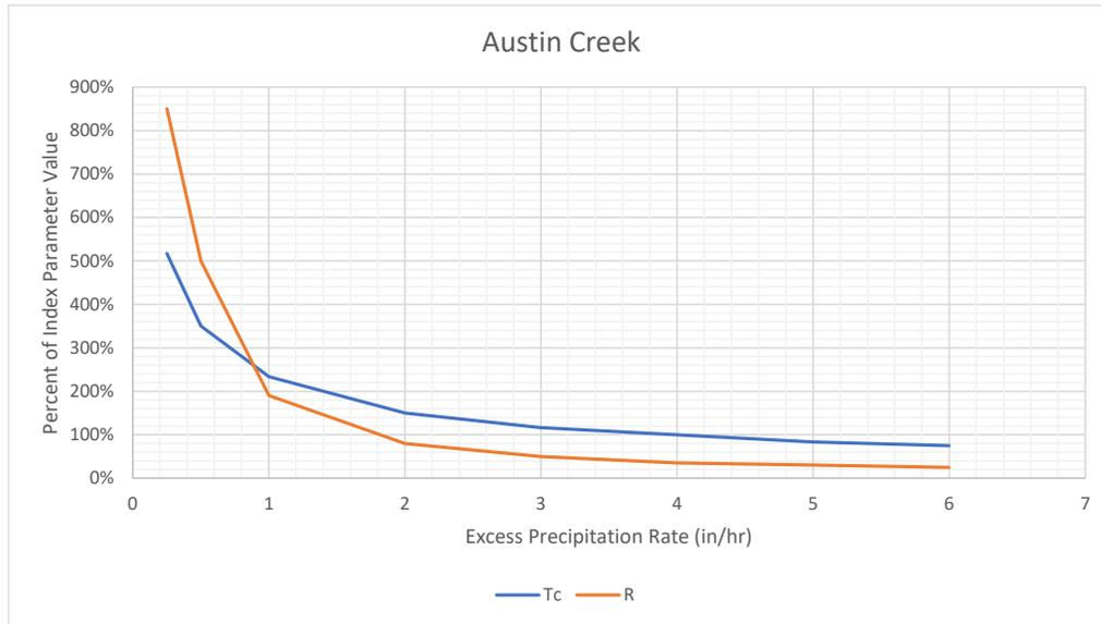
Figure 4. Example of Dimensionless Ratios of  $T_c$  and  $R$  Relative to Index Parameters for Austin Creek
