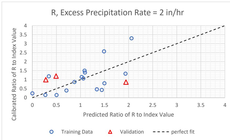
Figure 9. Excess Precipitation Rate = 2 in/hr: Ratio of  $R_{index}$  Validation Results
