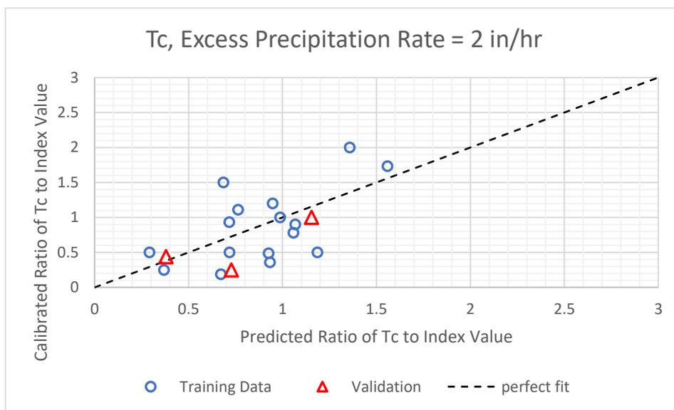
Figure 8. Excess Precipitation Rate = 2 in/hr: Ratio of  $T_{c,index}$  Validation Results
