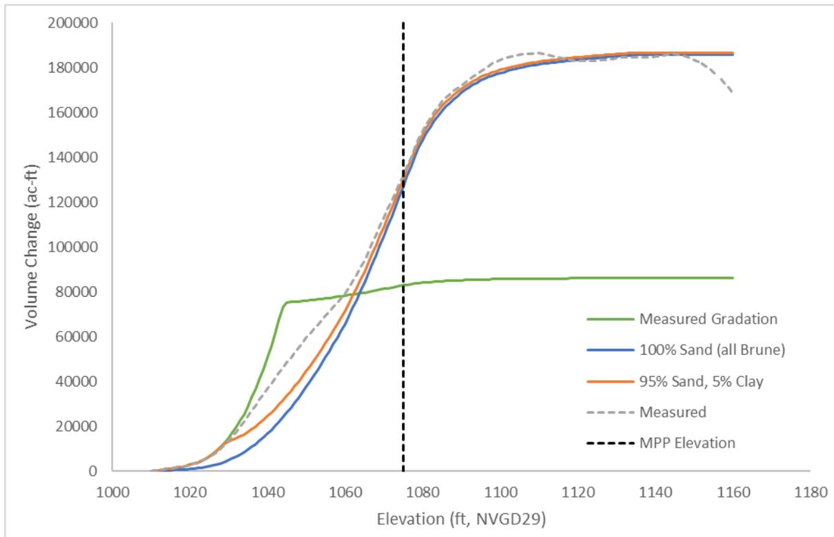
Figure 4: Measured and modeled volume change at Tuttle Creek (1972 to 2009)
