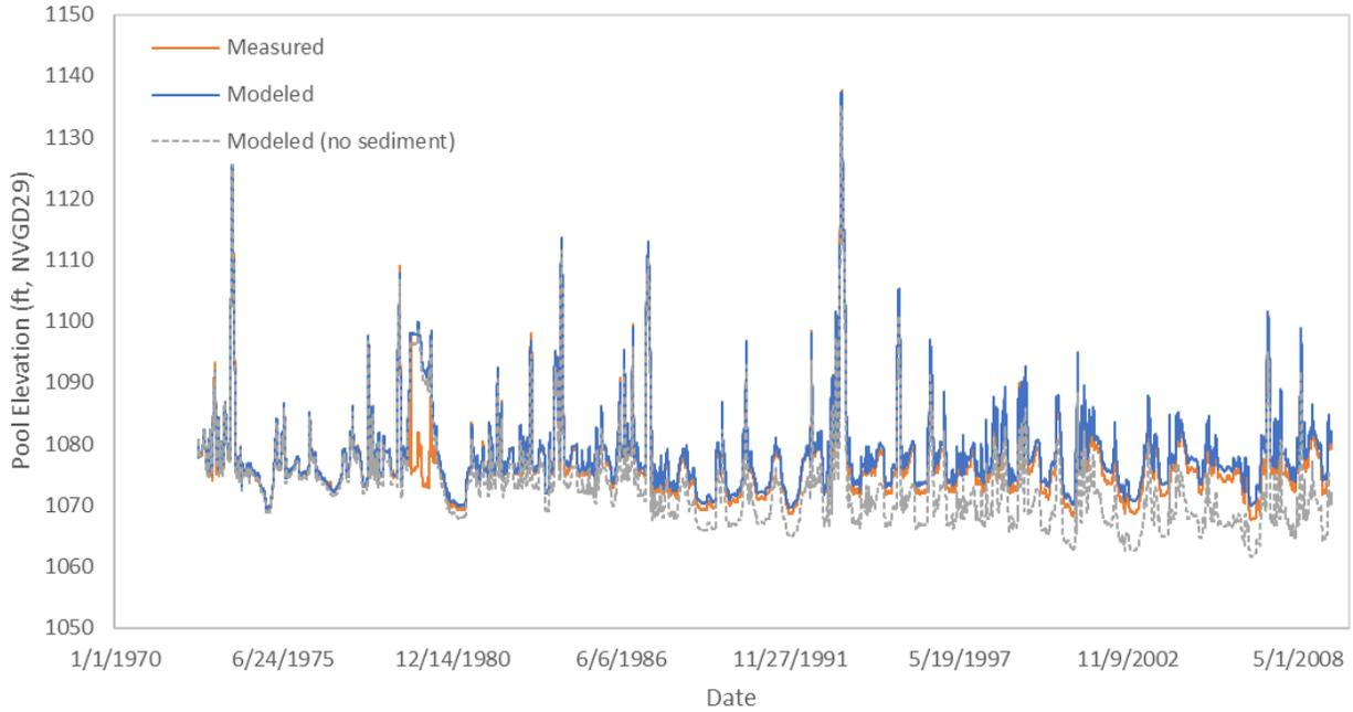
Figure 6. Measured and modeled pool elevation at Tuttle Creek
