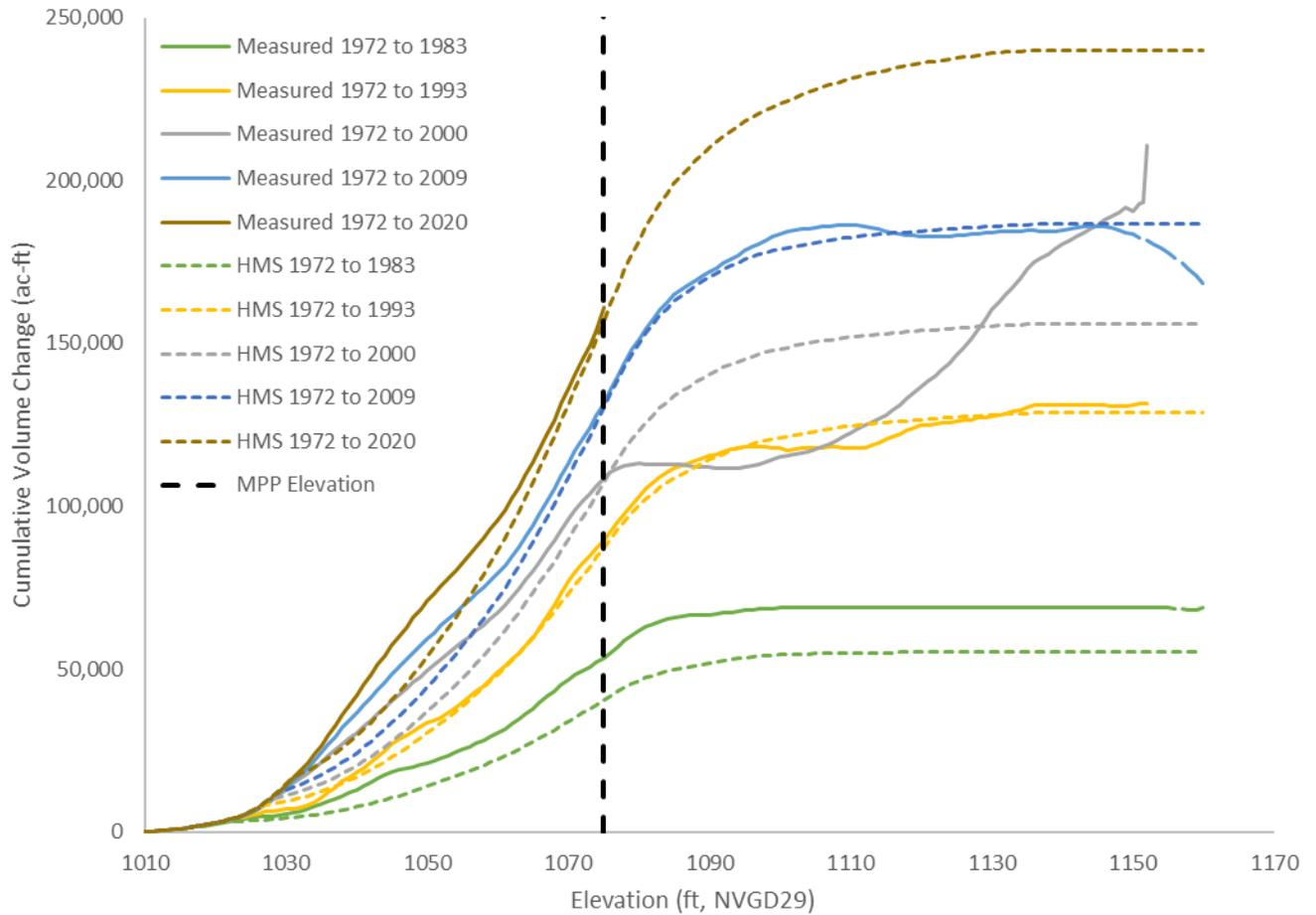
Figure 5. Tuttle Creek measured and modeled cumulative volume change relative to the 1972 survey
