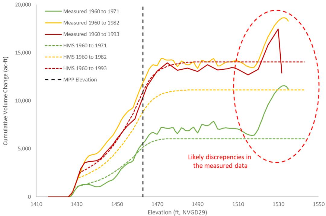
Figure 7: Kanopolis measured and modeled cumulative volume change relative to the 1960 survey
