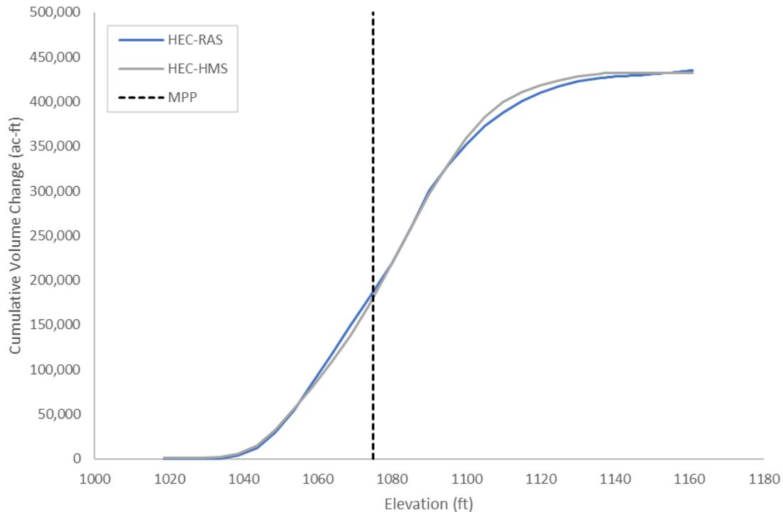
Figure 11: Projected FWOP volume change by elevation from 2024 to 2124
