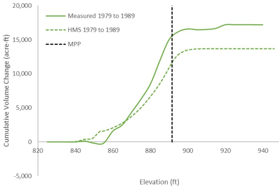
Figure 9: Perry measured and modeled cumulative volume change relative to the 1979 survey
