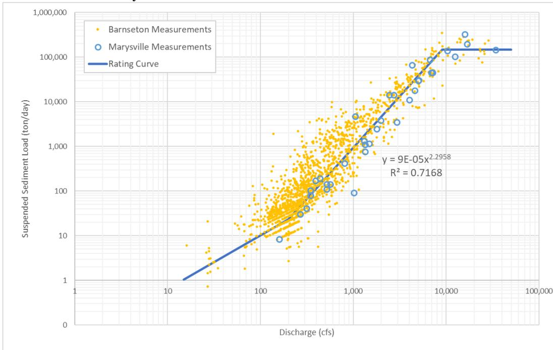
Figure 2. Example sediment rating curve used for computing daily sediment inflow
