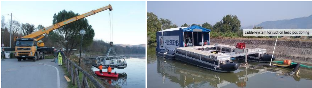
Figure 6: SediMover field test in 2nd reservoir
