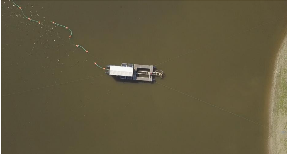
Figure 3: SediMover with visible cable connections to anchor points
