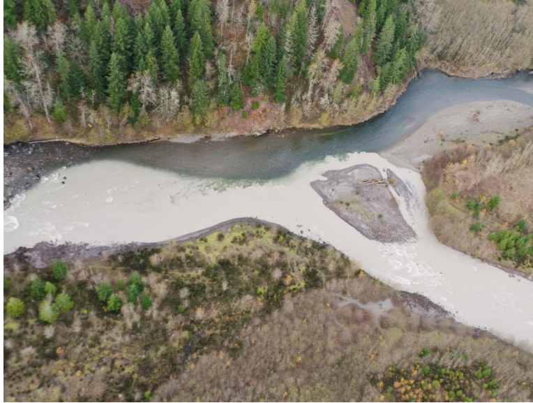
Figure 1. Natural color aerial photograph of North Fork Toutle River and Green River confluence showing water with high suspended-sediment concentration (light brown) mixing with clear tributary water.
