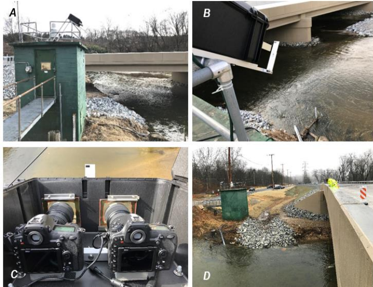
Figure 2. Field data collection panel showing (A) the ‘SedCam v2.0’ camera system mounted on a handrail on the gage house roof (view looking downstream toward bridge), (B) camera housing with white balance calibration card mounted underneath and pump sample intake on left bank, (C) interior of camera housing looking toward river surface, and (D) depth-integrated sampler deployed from the bridge.
