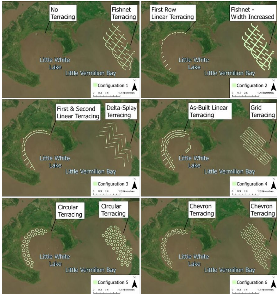
Figure 2. Model Configurations. The figure conceptualizes the shapes of the terrace configurations for each of the six model simulations.
