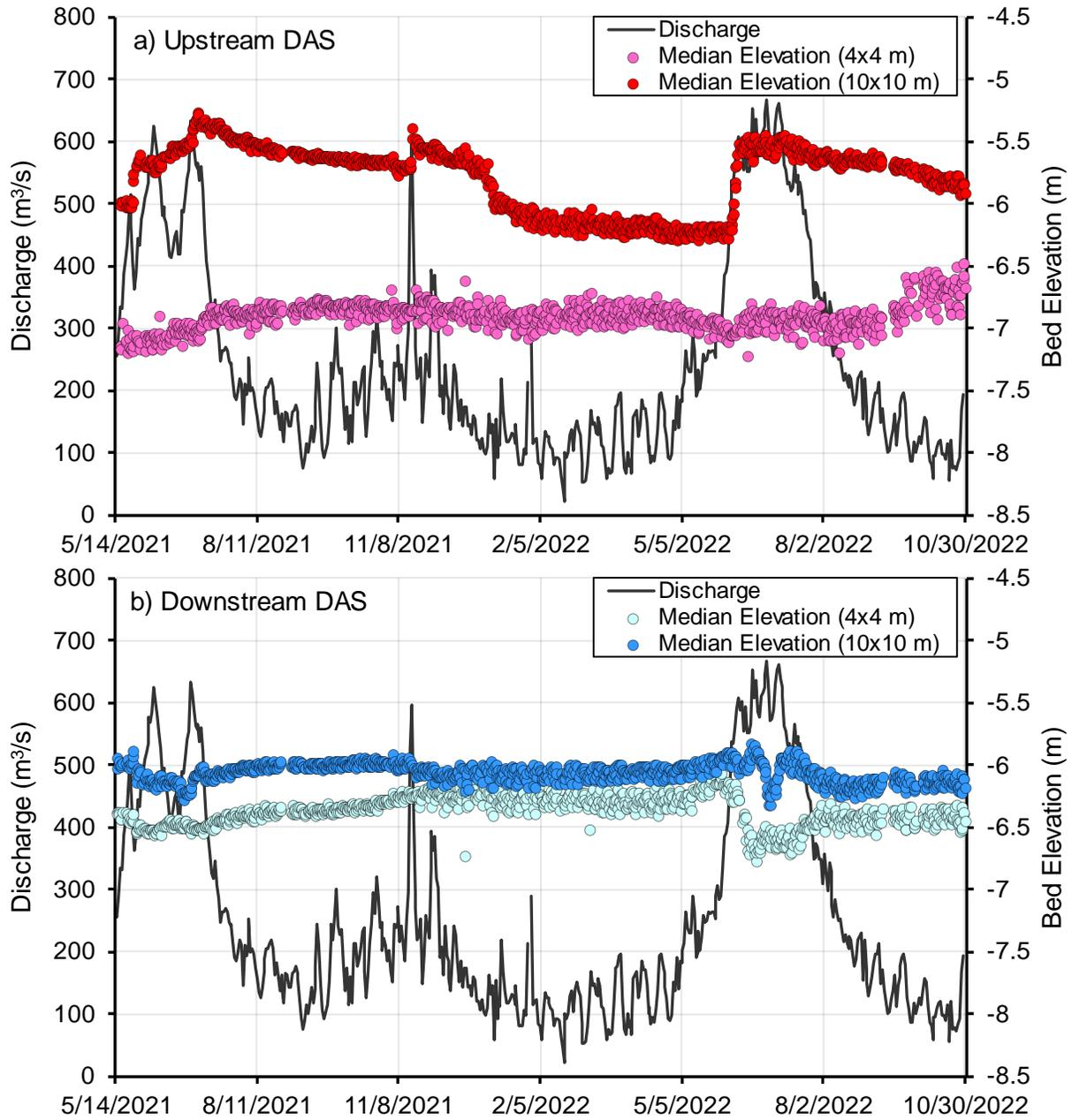
**Figure 3.** Median bed elevations extracted for each scan from the (a) upstream, and (b) downstream DAS, alongside the daily discharge record for the RSMS.
