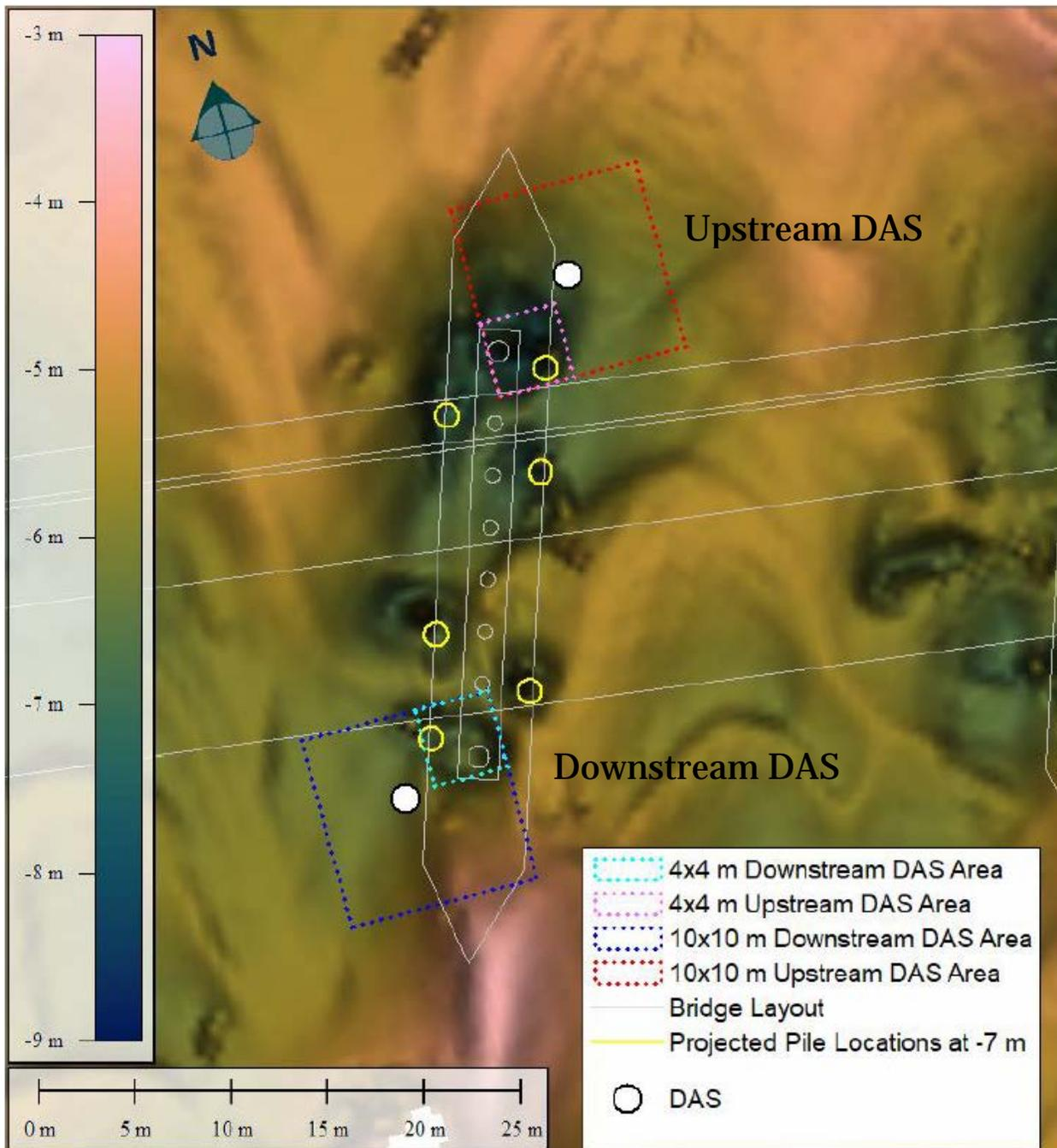
**Figure 2.** Location of grids used to examine bed elevation changes around the pier through time. Flow reverses at this site, but the landward to seaward direction is from top to bottom. Multibeam bathymetric survey shown in background was collected by NHC in February 2022. Elevations in Canadian Geodetic Vertical Datum of 1928.
