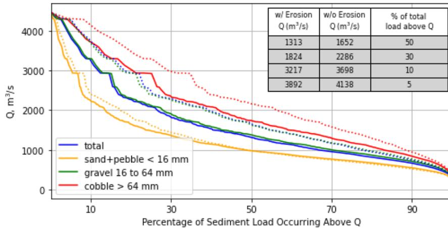
**Figure 3.** Dependence of cumulative sediment load on discharge for node at upstream coordinate 40 km. Solid lines denote simulation that includes bank erosion. Dotted lines denote simulation that does not include bank erosion.
