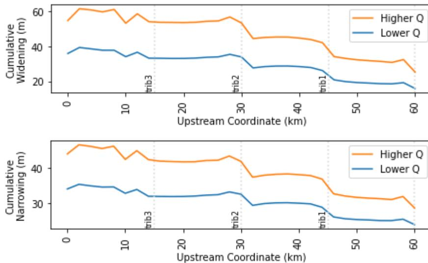
**Figure 2.** Cumulative widening and cumulative narrowing over the course of the simulation for base hydrology (denoted Lower Q) and invigorated hydrology 20% larger than base (denoted Higher Q). Tributary confluences are shown with the vertical dotted lines.
