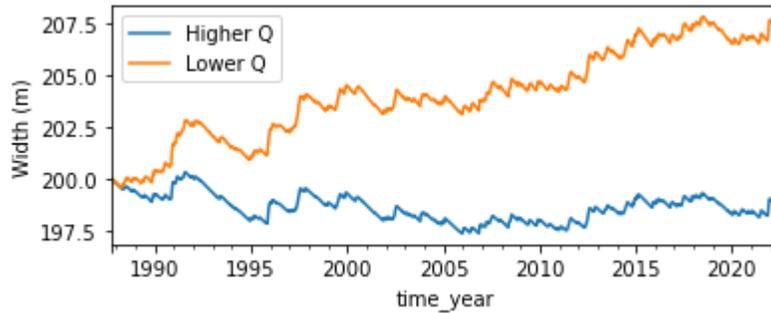
**Figure 1.** Simulated channel width at mid-reach node (at upstream coordinate 40 km).
