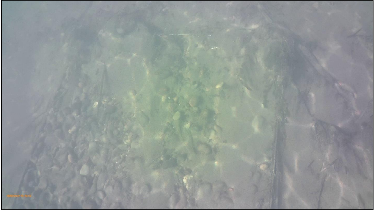
Figure 10. Underwater photo taken of the Offshore Sensor Array (Grid 1378) on October 3 rd , 2022, confirming that the increased heat signal was produced by infilling of the clean gravels with fine sediment
