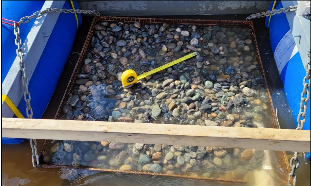
Figure 4. Temperature sensor array covered with clean gravel prior to deployment to mimic newly restored substrate
