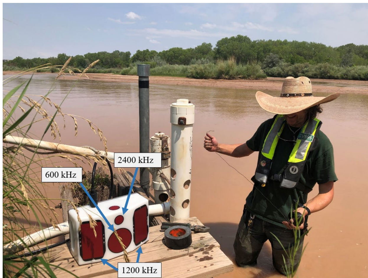
Figure 1. Temporary deployment of the Horizontal Acoustic Sediment and Current Profiler (HASCP) at the Rio Grande at Central, Albuquerque, NM (USGS ID 08330000) in July 2021. Tyson Hatch (U.S. Geological Survey) is shown here with the HASCP which was mounted to a solid aluminum pole and secured to existing infrastructure for 4 hours during operational testing. Maximum depth in the channel during deployment was approximately 3 feet.
