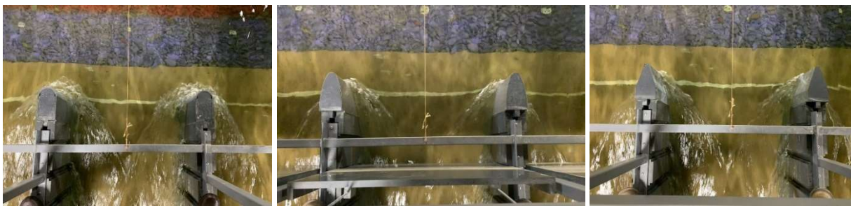
Figure 5. Pier nose shape alternatives tested in physical model: rounded (left), ellipse (middle), octagonal (right)
