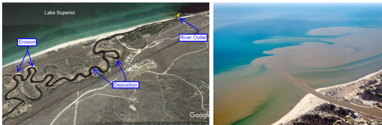
Figure 1. Examples of Deposition and Erosion Within a Fluvial System, Two Hearted River (61); Aerial Photograph Grand River Outlet (14) at Lake Michigan Following a Large Storm Event, April 22nd, 2013 (Beaver M, 2013)
