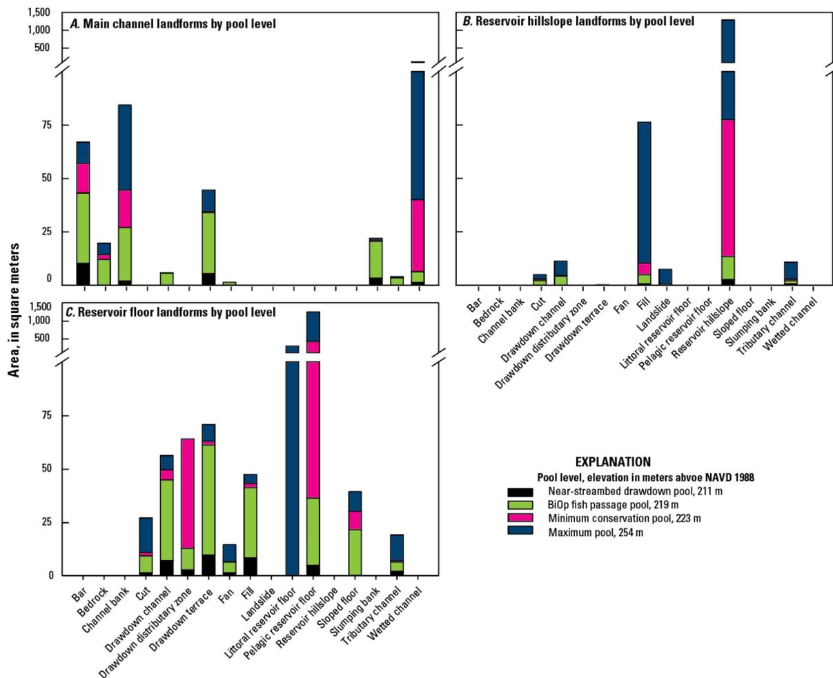
**Figure 4.** Graph of the distribution of mapped geomorphic landform units as a function of pool elevations at Fall Creek Lake, Oregon, for the A) main channel, B) reservoir hillslope, and C) reservoir floor mapping domains (data from Keith and Stratton Garvin, 2021, analyses show provisional data, subject to revision).
