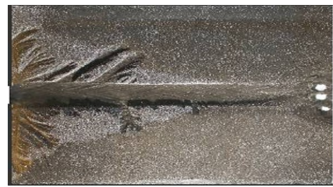
Fig 1. Channel networks in the reservoir in fully drawdown flushing (Hajhosaini 2008)
