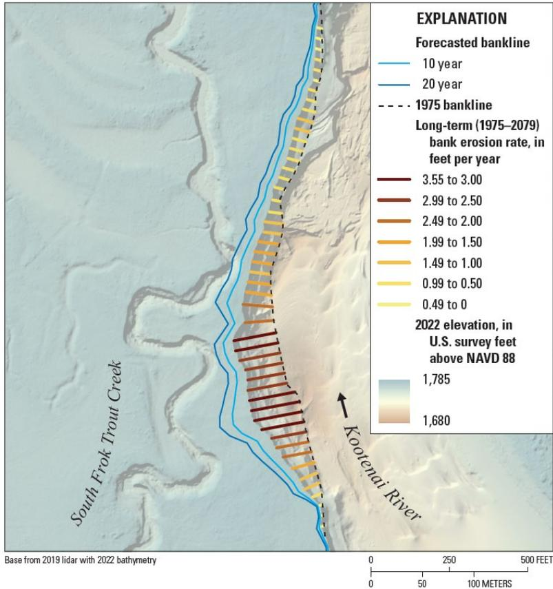
**Figure 4.** 10-year and 20-year forecasted banklines and long-term bank erosion rates near South Fork Trout Creek at Trout Creek Peninsula on the Kootenai River near Bonners Ferry, ID computed from 1975 to 2019 average bank erosion rates
