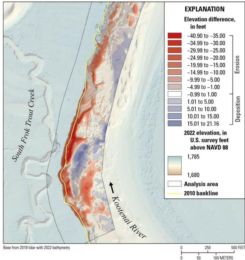
**Figure 6.** Digital elevation model (DEM) of difference between 2010 and 2022 showing areas of erosion and deposition near South Fork Trout Creek. Negative values (warmer colors) represent erosion and positive values (cooler colors) represent deposition
