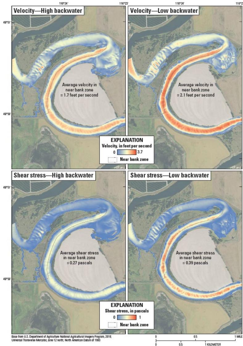
**Figure 7.** Simulated shear stress and depth averaged velocity at Trout Creek Peninsula for high flow conditions with significant backwater from Kootenay Lake (31,850 ft<sup>3</sup>/s on June 17, 2022) and high flow conditions with less backwater influence from Kootenay Lake (33,026 ft<sup>3</sup>/s on December 3, 2021)
