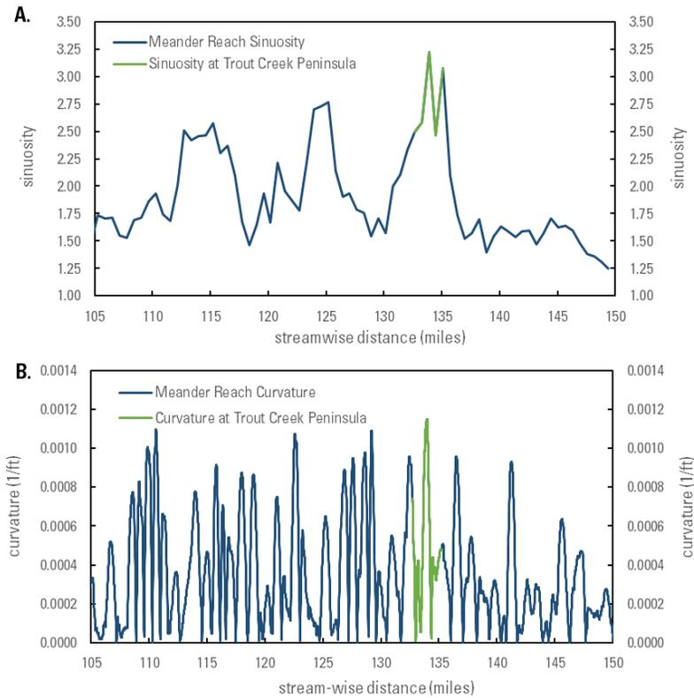
**Figure 3.** (A) Sinuosity and (B) curvature of the Kootenai River meander reach from Porthill, ID (river mile 105) to Ambush Rock (river mile 152)
