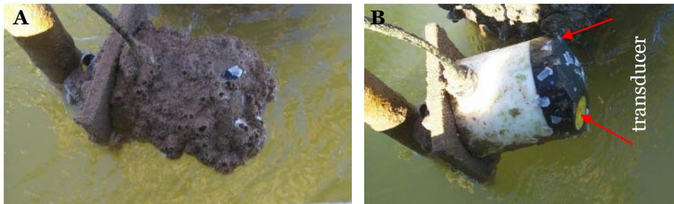
**Figure 3.** Photographs of an acoustic Doppler velocity meter *A*, before cleaning and *B*, after cleaning the instrument for barnacles; the transducers used to measure the acoustic backscatter signal are identified in panel B (photographs taken by U.S. Geological Survey)
