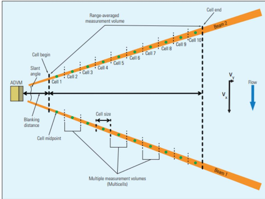
**Figure 2.** Generalized measurement volumes for a side-looker acoustic Doppler velocity meter (reprinted from Levesque and Oberg, 2012 [fig. 8])
