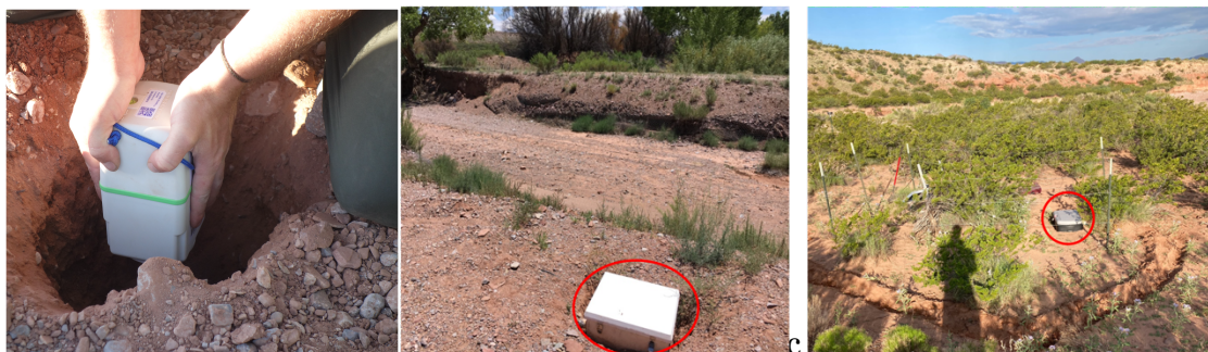
Figure 3: Installation of a seismic node (left) and two types of broadband seismometers deployed adjacent to the ADLP. Broadband sensors are buried underground, with surface vaults (red circle) housing the data loggers and other electronics.
