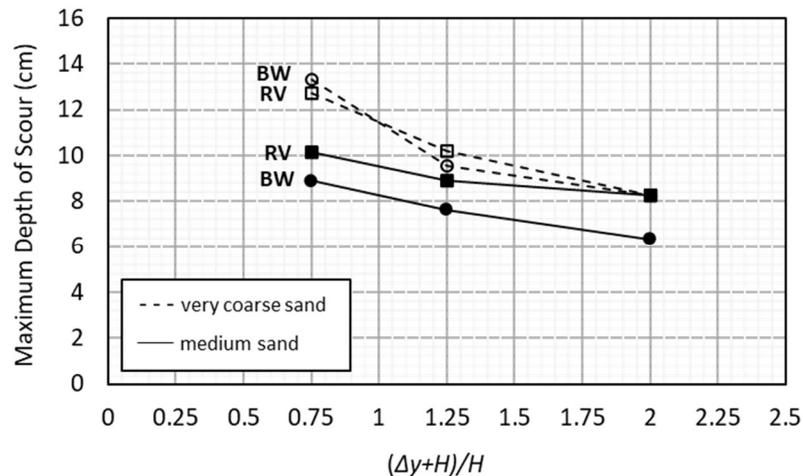
**Figure 9.** Maximum depth of scour versus  $(\Delta y+H)/H$  for bendway weirs (BW) and rock vanes (RV) on beds of very coarse sand or medium sand.
