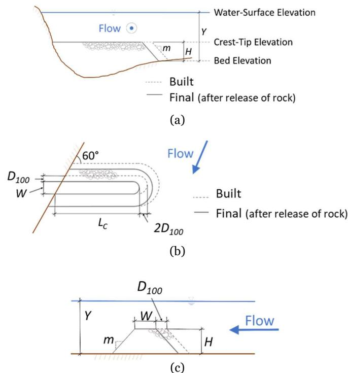
**Figure 11.** Recommendation for the design of a bendway weir: (a) streamwise, cross-section view of the design recommendation; (b) plan view of the design recommendation (widened for the upstream rock structure only); and (c) centerline elevation view (looking toward outer bank) of the design recommendation. A design alternative is to face the tip of final shape with a double layer of rock larger than the median size of rock used to build the bendway.
