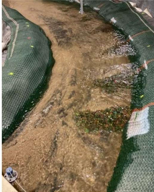
**Figure 4.** View of the curved flume fitted with six bendway weirs on the bed of medium sand, and  $(\Delta y + H)/H \approx 1.25$
