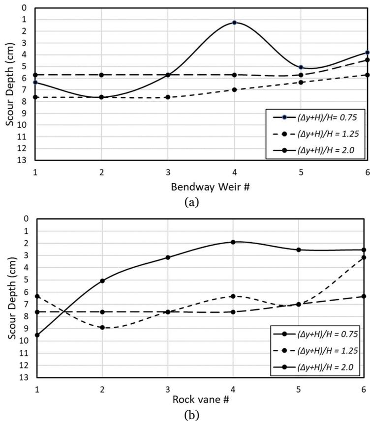
**Figure 8.** Scour depth at tips of bendway weirs and rock vanes on very coarse sand: (a) bendway weirs; and (b) rock vanes. Structures are numbered from upstream to downstream (see Figure 5).
