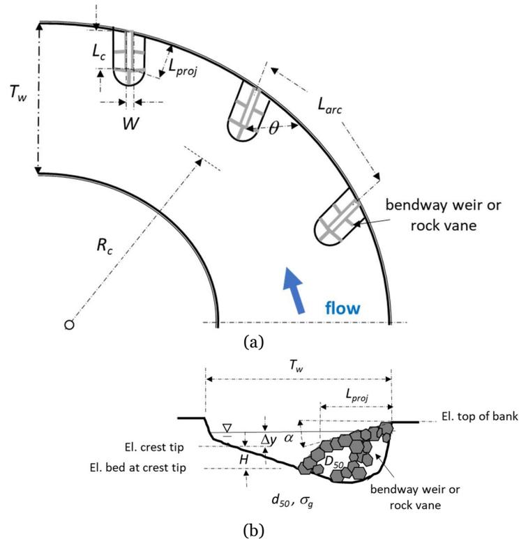
**Figure 3.** Variables used for the dimensional analysis leading to Equation (1). The indicated flow direction concurred with the direction used for the experiments.
