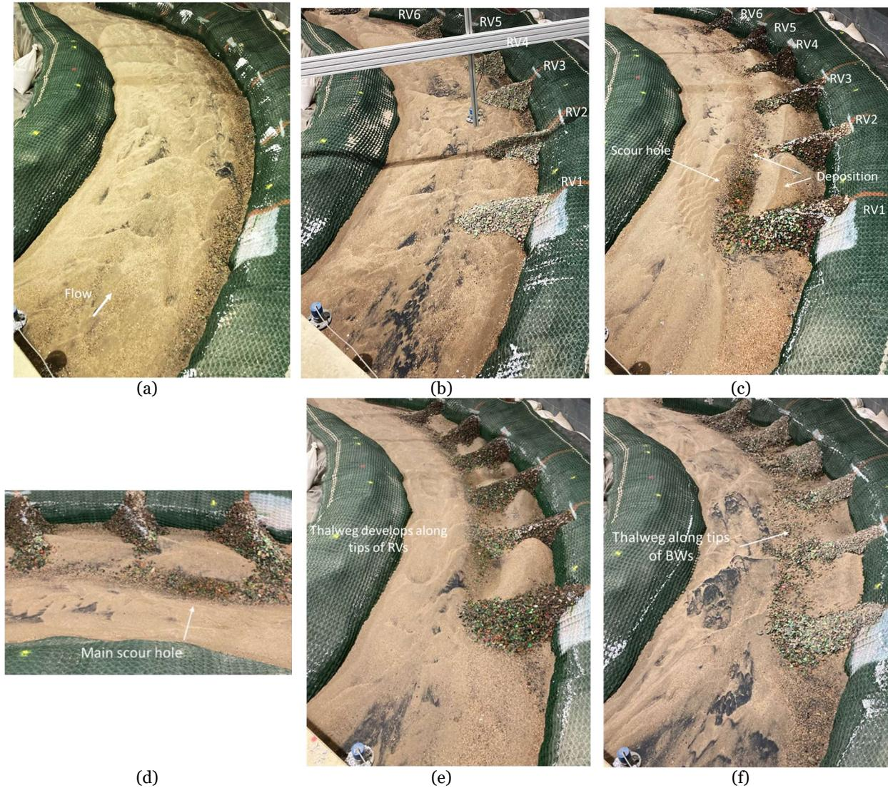
**Figure 5.** Scour, thalweg development, and failure modes of six rock vanes on the bed of very coarse sand: (a) no rock vanes,  $Q = 2.5$  cfs ( $0.07 \text{ m}^3/\text{s}$ ); (b) newly built rock vanes before experiment; (c)  $(\Delta y + H)/H \approx 0.75$  (after experiment); (d) a detail view of (c); (e)  $(\Delta y + H)/H \approx 1.25$  (after experiment); (f)  $(\Delta y + H)/H \approx 2.0$  (after experiment)
