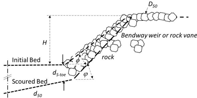
**Figure 10.** Scour at the toe of a rock pile may destabilize the toe; scour depth at toe =  $d_{s-toe}$ . Here,  $\alpha$  = built slope of tip face, and  $\phi$  = equilibrium slope of rock loosely piled. This figure assumes no crossflow of water across the tip face
