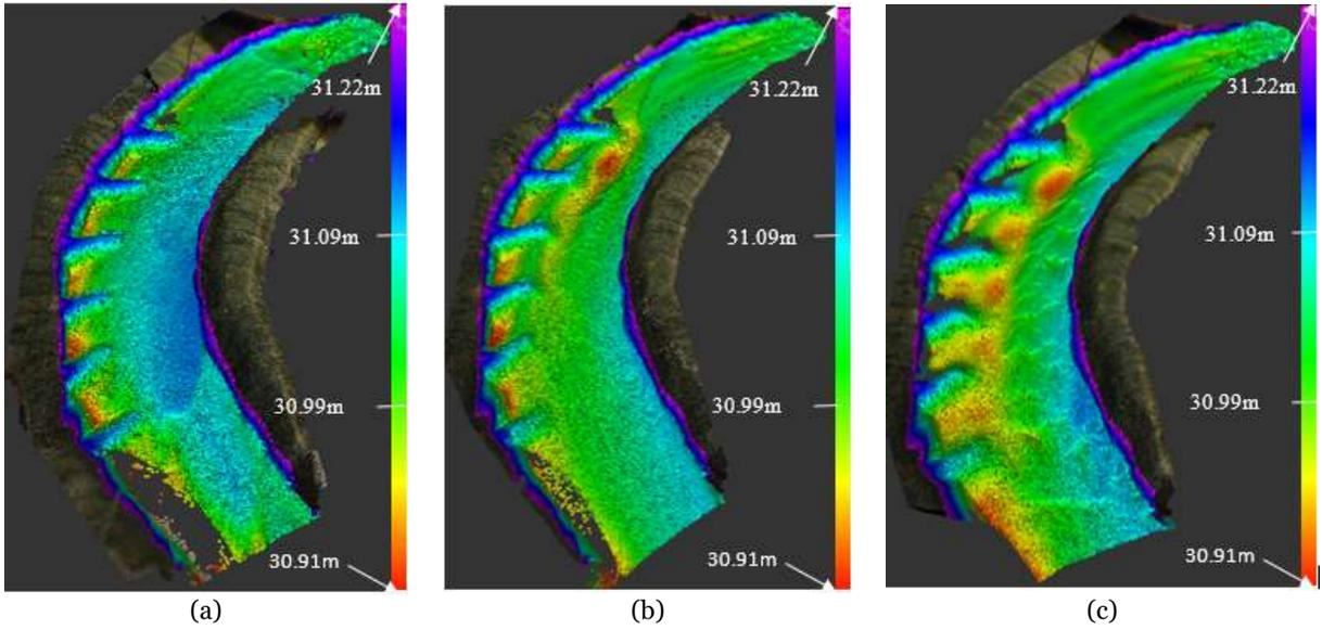
**Figure 7.** LiDAR scans for six bendway weirs on the bed of very coarse sand in the curved flume under the following flow-hydrograph conditions: (a) initial bed formed for  $(\Delta y+H)/H \approx 1.25$  and with bendway weirs newly placed; (b)  $(\Delta y+H)/H \approx 0.75$ ; and (c)  $(\Delta y+H)/H \approx 1.25$  (1.00 m  $\approx$  3.28 ft)
