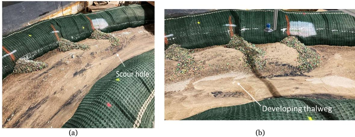
**Figure 6.** Scour region observed for the six bendway weirs: (a)  $(\Delta y+H)/H \approx 0.75$ ; and (b)  $(\Delta y+H)/H \approx 1.25$
