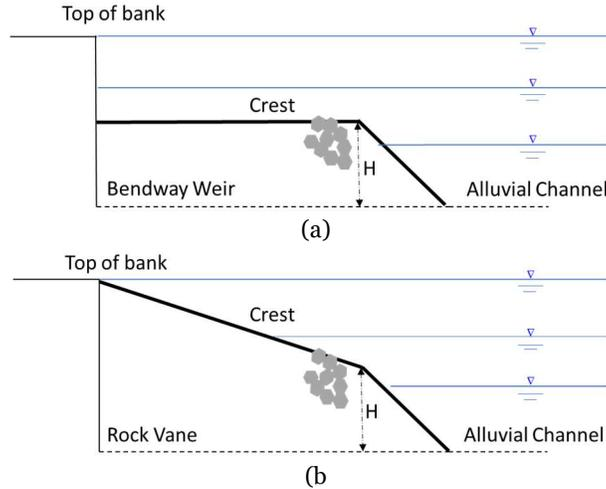
**Figure 2.** Cross-section profiles of (a) bendway weirs; and (b) rock vanes. These two profiles are transverse across channel and reflect the main difference between the two rock structures. Three flow depths are indicated.
