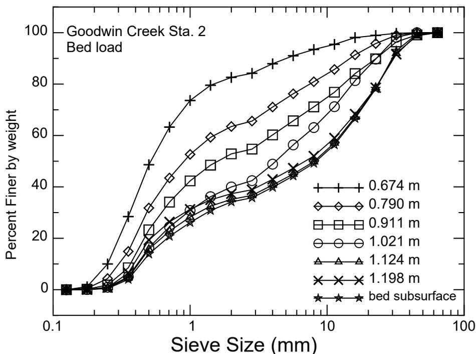
**Figure 3.** Mean grain size distributions of bed load from samples collected during 1984-1988 at structure 2, GCEW.
