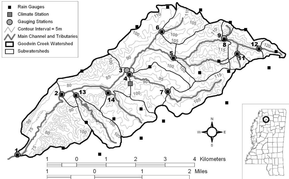
**Figure 1.** Map of GCEW with elevation contours, gauging station locations and rain gauge locations.
