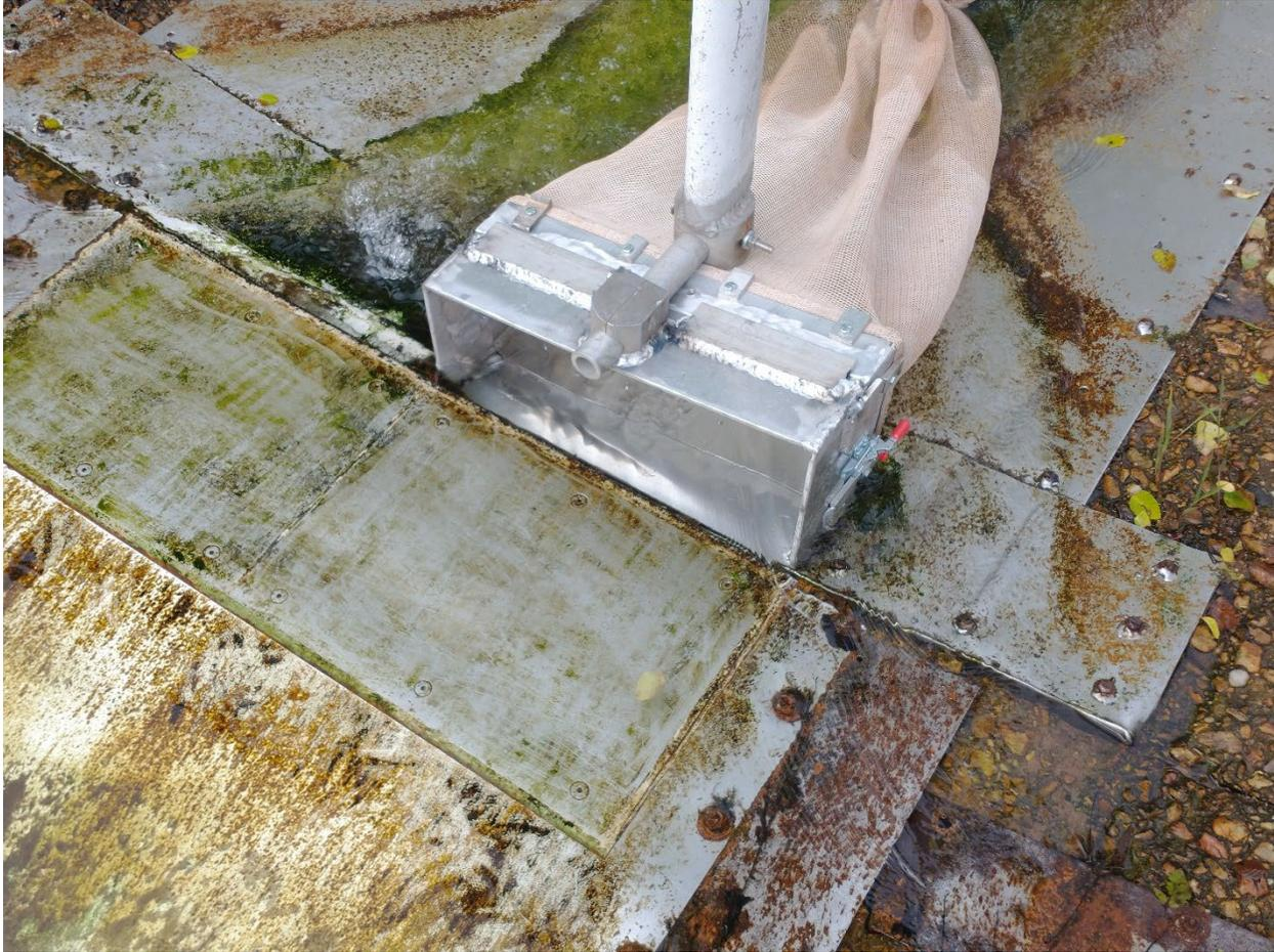
**Figure 4.** Impact plates with bed-load trap sampler in position just downstream of one of the plates. Photo taken at base flow.
