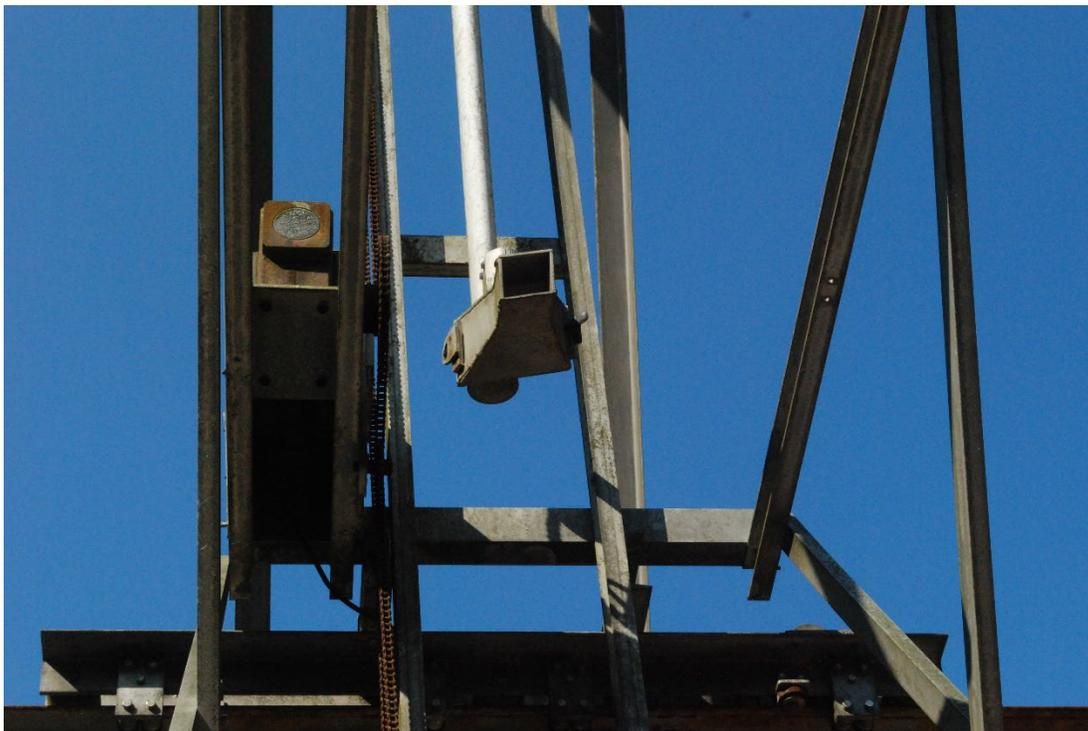
**Figure 2.** (Top) Upstream footbridge and sampling rig at station 3 of GCEW. (Bottom) Closeup of modified Helley-Smith sampler on sampling rig at station 3. The sampling equipment at structure 3 is very similar to that at station 2.
