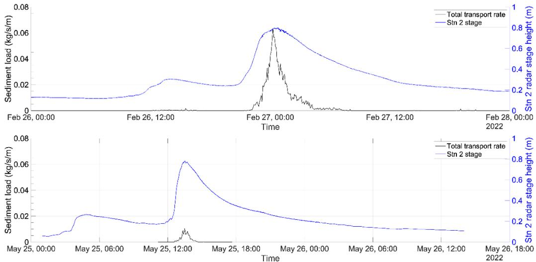
**Figure 6.** Stage and bed-load transport rate from May 25, 2022, and February 27, 2022 runoff events. Peak flow depth at the measurement station was 0.78 and 0.80 m for the May 25 and February 27 events, respectively.
