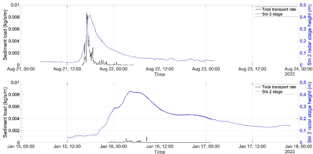
**Figure 5.** Stage and bed-load transport rate from January 16, 2022, and August 21, 2022 runoff events. Peak flow depth at the measurement station was 0.43 and 0.42 m for the January 16 and August 21 events, respectively.
