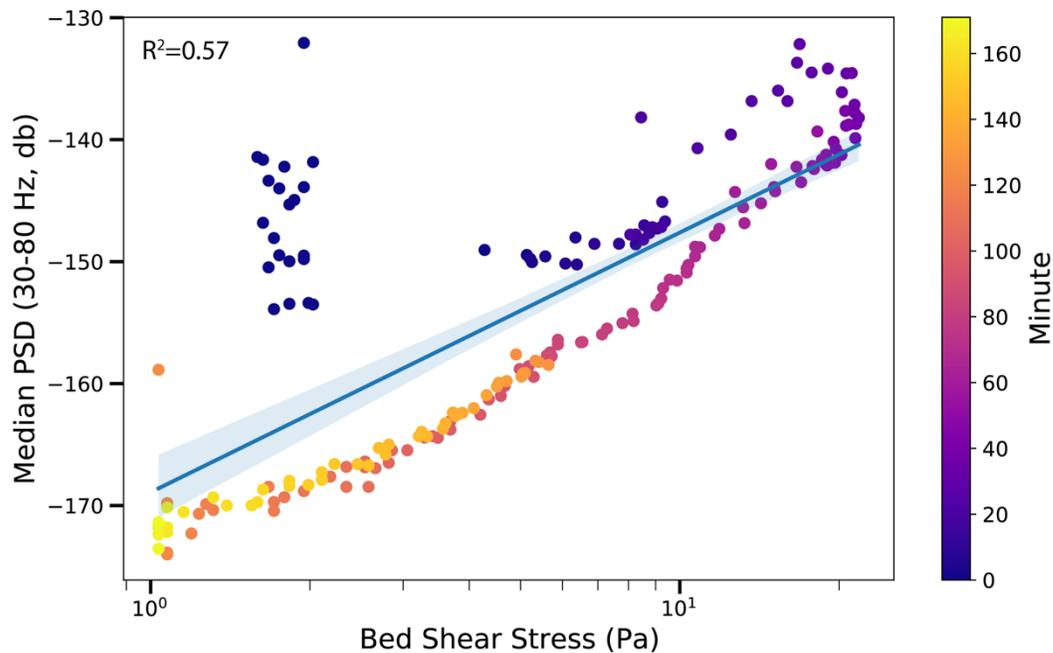
**Figure 4.** Median seismic PSD within the 30-80 Hz frequency band as a function of calculated bed shear stress during the 2021-08-23 09:00-13:00 UTC flood event using data from seismic station GBB. Circles are colored by minute following the start of water depth measurement. Best fit regression line included (blue line) with 95% confidence interval (blue shading).
