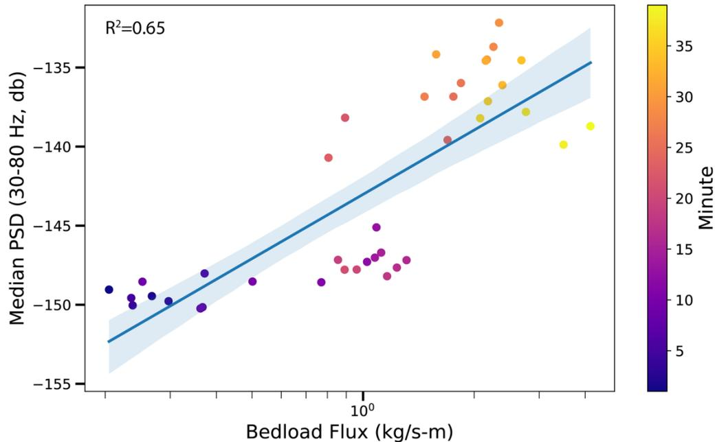
**Figure 3.** Median seismic PSD within the 30-80 Hz frequency band as a function of measured bedload flux during the 2021-08-23 09:00-13:00 UTC flood event, using data from station GBB. Circles are colored by minute following the start of bedload flux measurement; note this is only a small portion of the overall flood duration shown in Figure 2. Best fit regression line included (blue line) with 95% confidence interval (blue shading).
