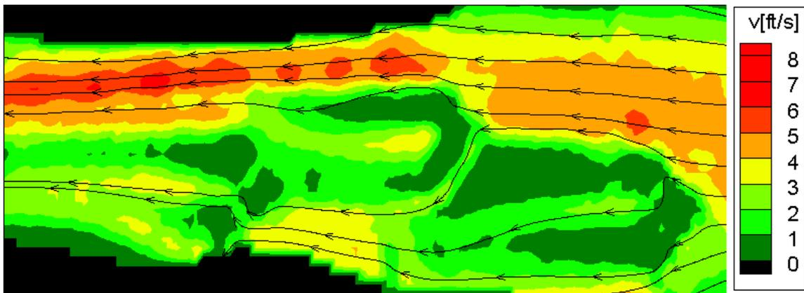
**Figure 8.** TecPlot output for velocity at 300 cfs at the upstream “V”, medium density configuration. Desired resting areas (< 3 ft/s) are denoted in green. Black spaces denote areas too shallow for analysis and were masked in PIVLab. For more results, please see Holste et al. 2019.
