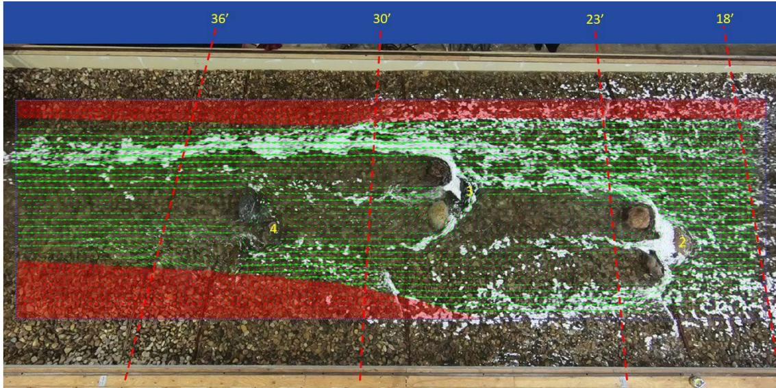
**Figure 7.** PIVLab output of velocity vectors at 300 cfs at the upstream “V”, medium density (or 3 cluster) configuration through the channel. Baseline ADV measurement transects are indicated with dotted lines, rock cluster numbers are denoted in yellow (2, 3, 4). Cluster 1 was removed for the medium density configuration. Red areas are “masked” portions that are either too shallow or too reflective for analysis in PIVLab. For more results, please see Holste et al. 2019.
