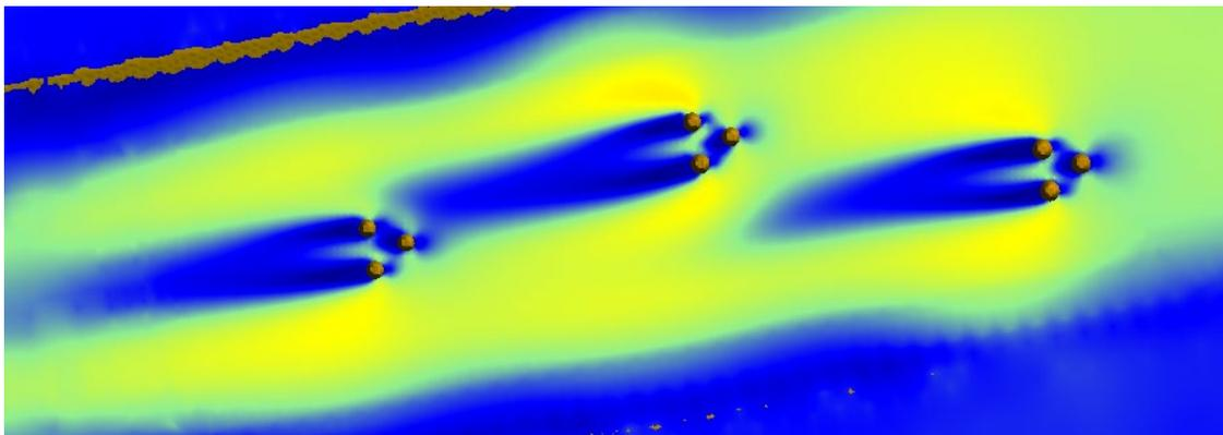
**Figure 9.** Numerical model velocity output at 300 cfs at the upstream “V” medium density configuration. Darker blue colors represent lower velocity while brighter yellow represents higher velocity. For more results, please see Holste et al. 2019.
