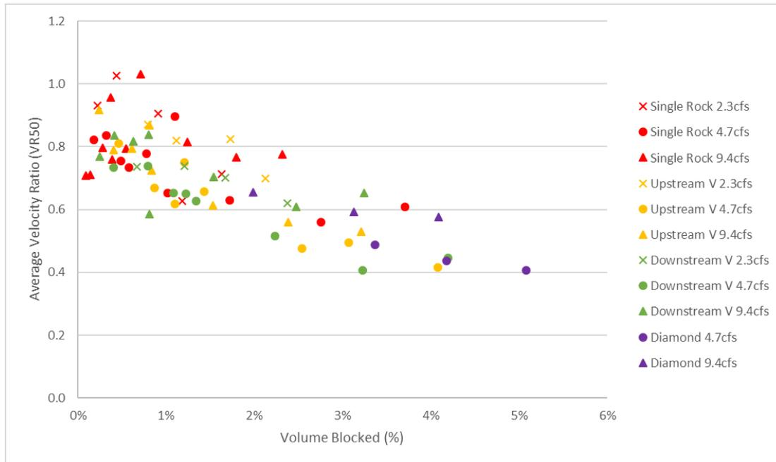
**Figure 14.** Percent volume blocked for every configuration and average velocity ratio. The average velocity ratio is the average velocity per test taken with respect to the corresponding baseline average velocity for each flow rate. Each configuration represents both small and large rock tests. For more results, please see Shinbein and Holste 2020.
