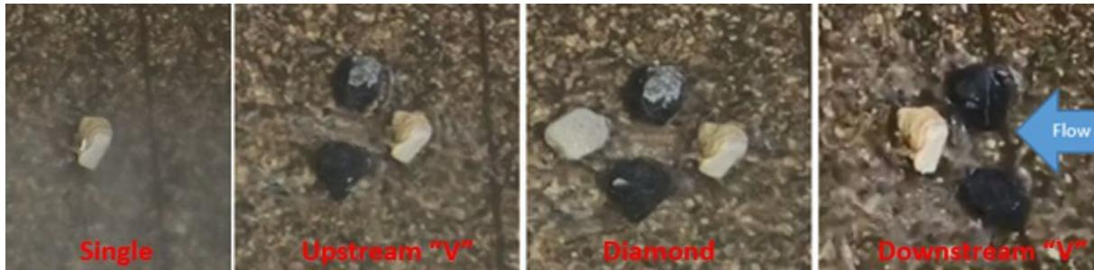
**Figure 3.** Single, upstream “V”, diamond, and downstream “V” configurations, respectively for the large boulder tests. For the small boulder tests only the single, upstream “V”, and downstream “V” configurations were tested. For more information, please see Holste et al. 2019.
