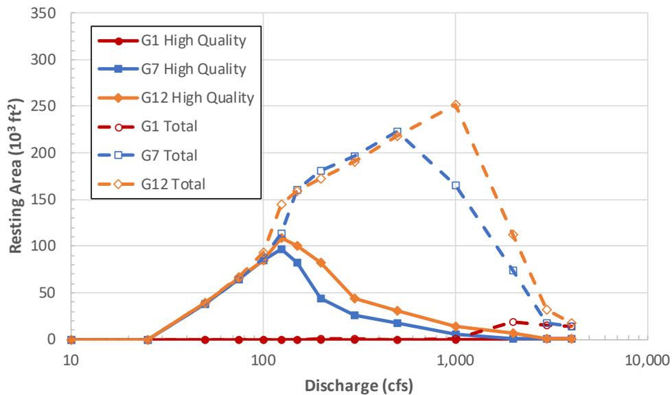
**Figure 10.** Comparison of high quality and total resting area for three geometry scenarios: existing conditions (G1), a roughened meandering pool-riffle channel (G7), and boulder clusters (G12). For more results, please see Holste et al. 2019.
