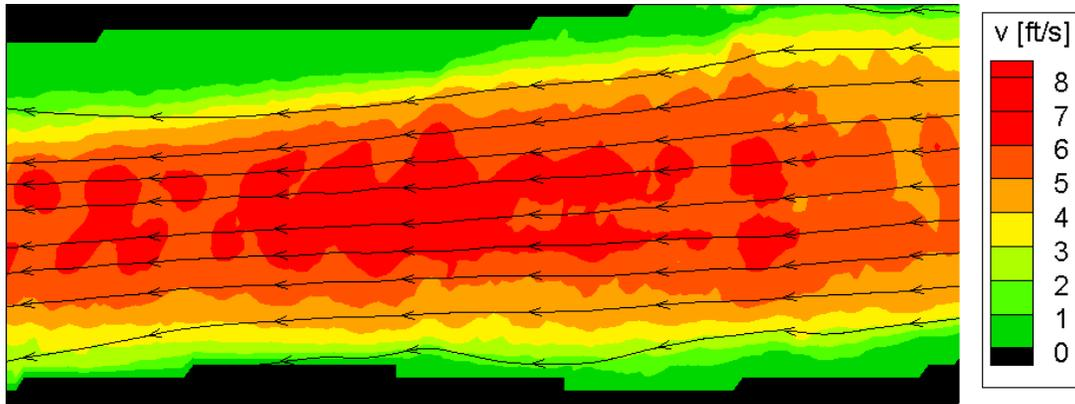
**Figure 5.** TecPlot output for velocity at 300 cfs baseline flow through the channel. Desired resting areas ( $< 3$  ft/s) are denoted in green. Black spaces denote areas too shallow for analysis and were masked in PIVLab. For more results, please see Holste et al. 2019.
