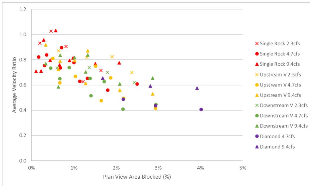
**Figure 12.** Percent plan view area blocked for every configuration and average velocity ratio. The average velocity ratio is the average velocity per test taken with respect to the corresponding baseline average velocity for each flow rate. Each configuration represents small and large rock tests. For more results, please see Shinbein and Holste 2020.
