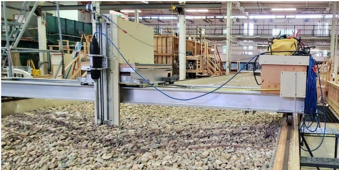
**Figure 2.** ADV mount in the physical model. The ADV can move horizontally and laterally along length and width of the model. For more information on data collection methods, please see Holste et al. 2019.
