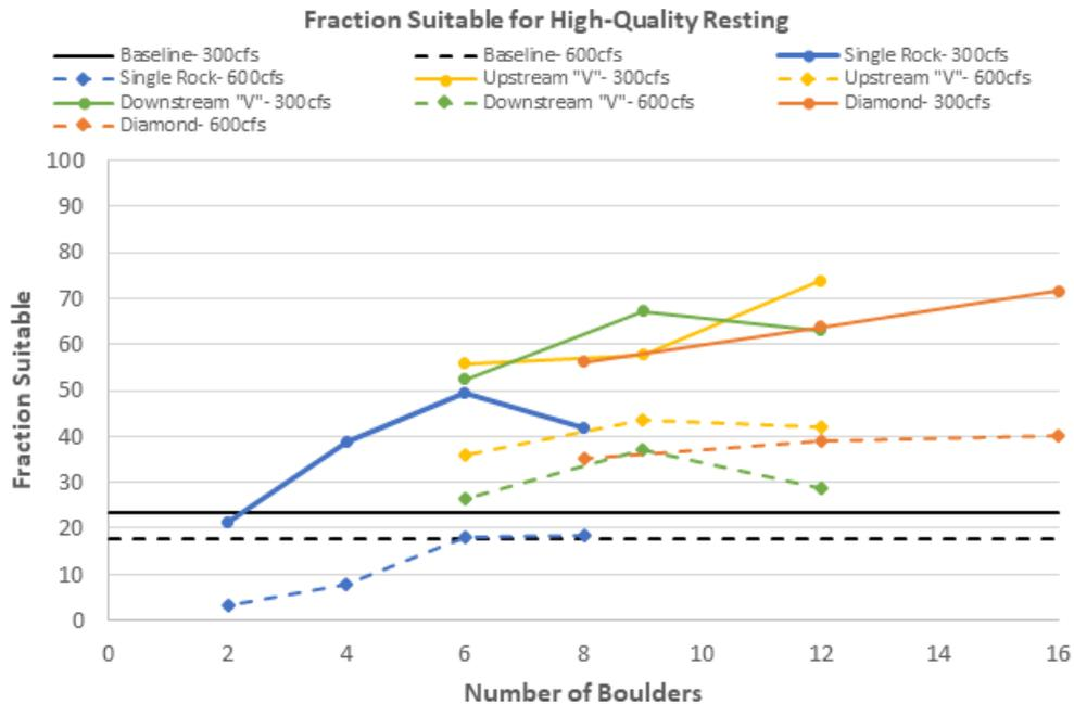
**Figure 6.** Fraction suitable for high-quality resting ( $< 3$  ft/s) versus number of boulders for both flow rates tested (300 and 600 cfs, prototype). All 300 cfs are denoted in solid lines. For more discussion on the configurations not presented in this paper, see Holste et al. 2019.
