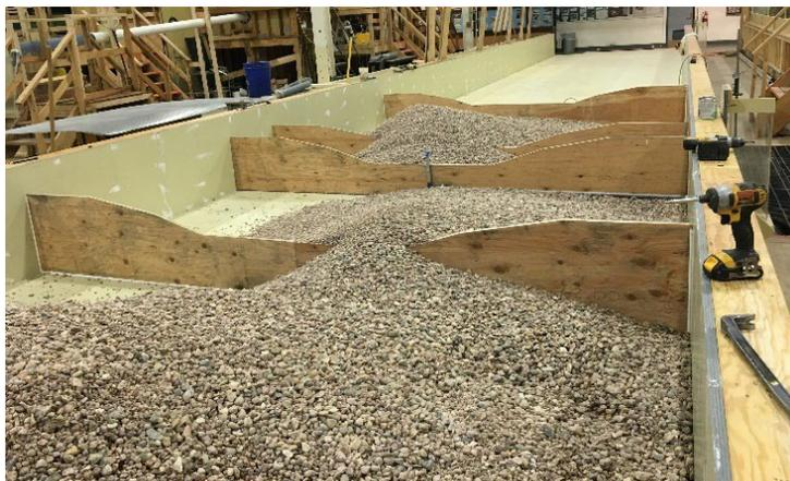
**Figure 1.** Template system used in model construction. For more information, please see Holste et al. 2019.
