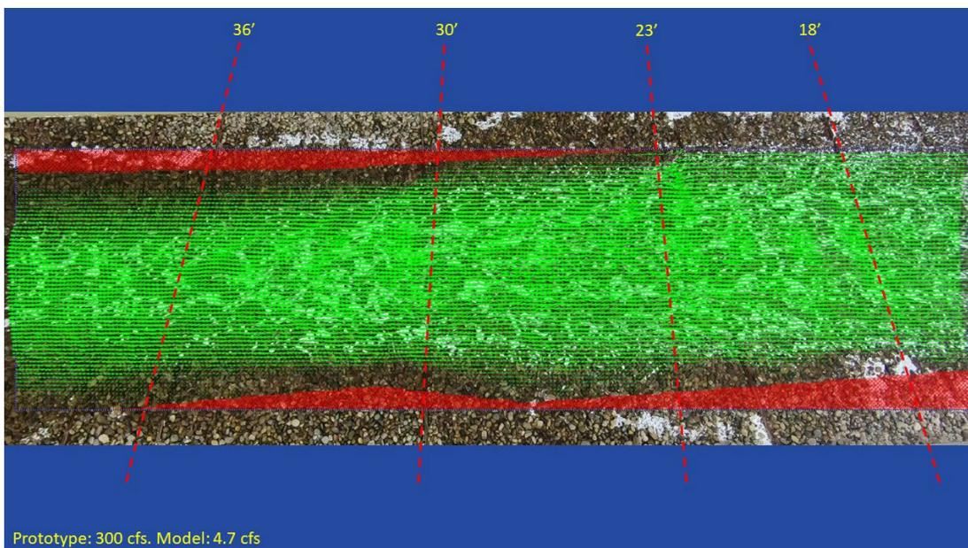
**Figure 4.** PIVLab output of velocity vectors at 300 cfs baseline flow through the channel. Baseline ADV measurement transects are indicated with dotted lines. Distances marked in figure represent offset downstream from the start of the model. Red areas are “masked” portions that are either too shallow or too reflective for analysis in PIVLab. For more results, please see Holste et al. 2019.
