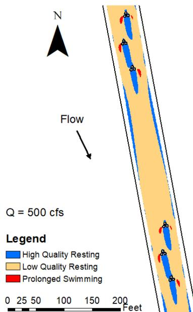
**Figure 11.** Velocity classification at 500 cfs for upstream V boulder clusters. Depths less than 1 ft are not shown. For more results, please see Holste et al. 2019.
