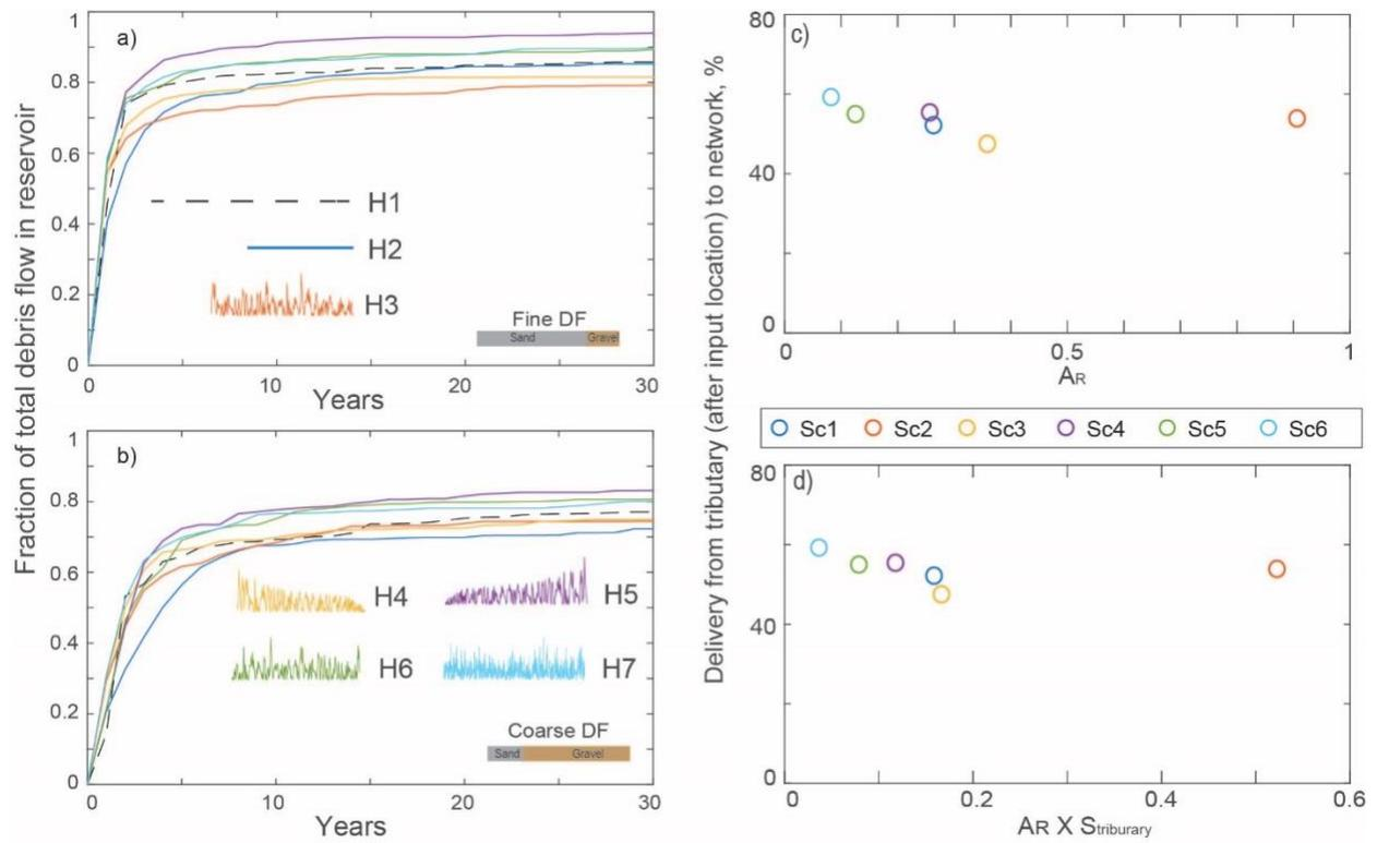
**Figure 2.** Debris flow sediment transported by all hydrographs for (a) fine and (b) coarse debris flow input. Percentage of input sediment (excluding the input location, gray area in Figure 3) delivered to mainstem after the 30-year simulation against (c) symmetry ratio ( $AR = DA_{tributary} / DA_{mainstem}$ ), and (d) product of symmetry ratio and tributary slope.
