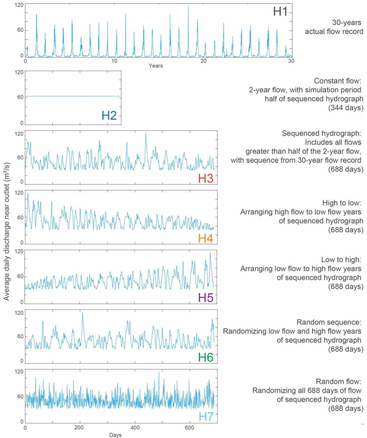
**Figure 1.** Construction of different hydrographs: H1 to H7. The discharge values are shown for USGS gage 10155000 (near basin outlet). The arranging of H4-H6 take average one-year segments of H3 when reordering/rearranging.
