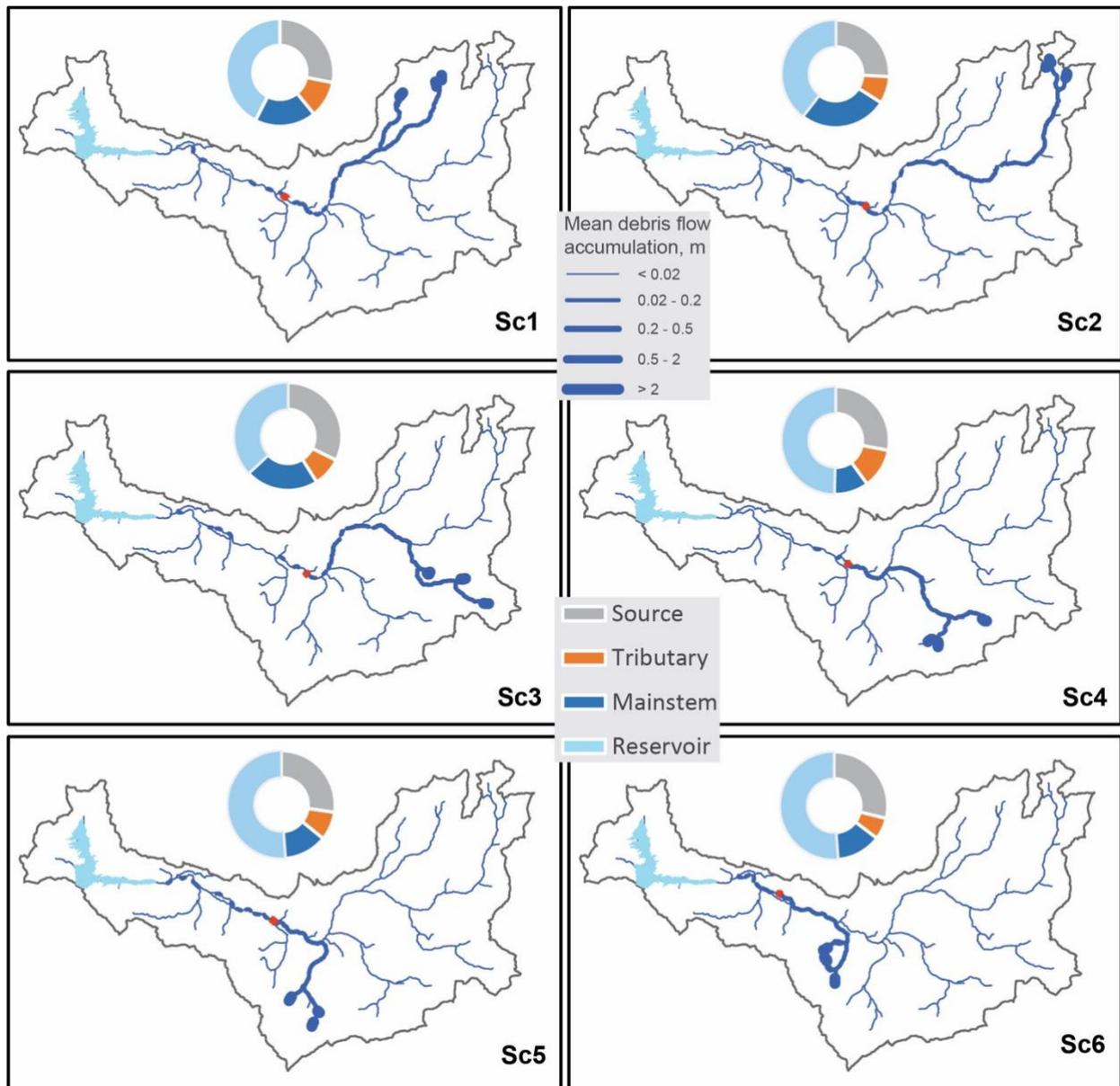
**Figure 3.** Debris flow accumulation in the Provo River network after the equivalent 30-yr flow simulation under different spatial input distributions (Sc1 to Sc6; initial placement at upstream tributary reaches). The proportions (of total 30,000 m<sup>3</sup>) of storage in the source location, tributary, mainstem and reservoir are shown by different colors in the circle. The downstream extent of 50% mainstem accumulation is showed by a red mark in the mainstem for each case.
