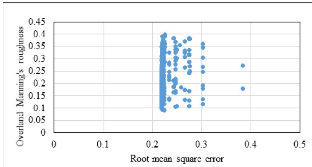
**Figure 11.** Manning's roughness versus Root Mean Square Error (RMSE) optimization based on SCE optimization algorithm.
