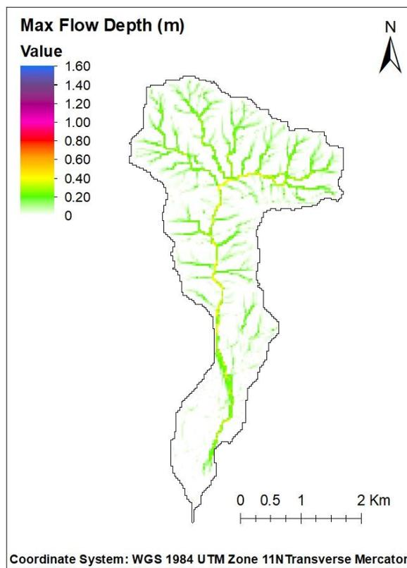
**Figure 5.** Pre-fire condition without considering the fire effects.
