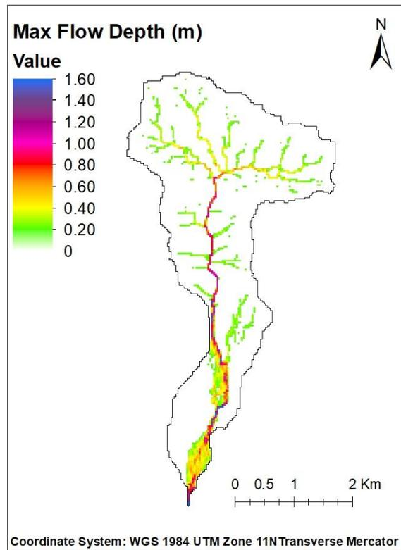
**Figure 7.** Post-fire infiltration condition with a reduction in soil hydraulic conductivity.
