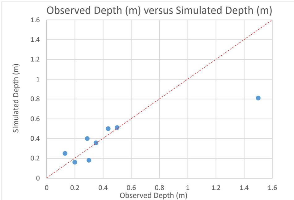
**Figure 9.** Observed depth versus simulated depth for the San Ysidro Creek of 09 January 2018 flows.
