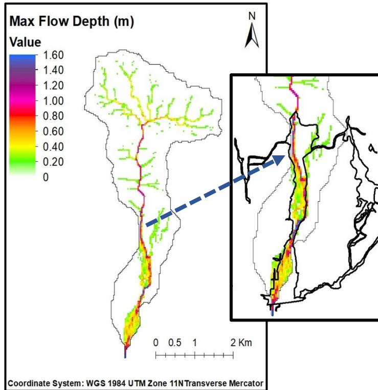
**Figure 8.** Simulated post-fire infiltration condition compared to observed maximum flow depths.
