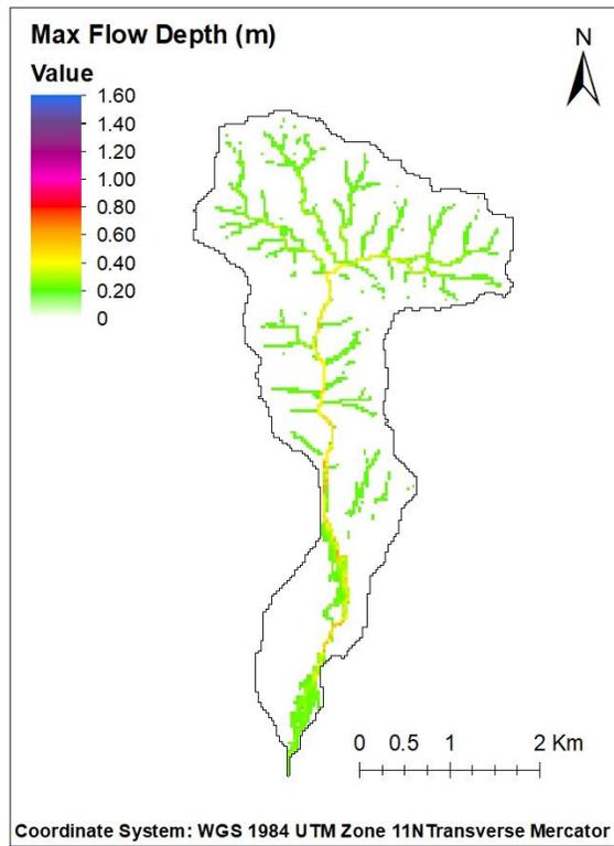
**Figure 6.** Post-fire routing condition developed with change in surface roughness.
