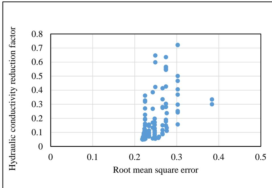
**Figure 10.** Hydraulic Conductivity Reduction Factor ( $R_{fk}$ ) versus Root Mean Square Error (RMSE) optimization based on SCE optimization algorithm.
