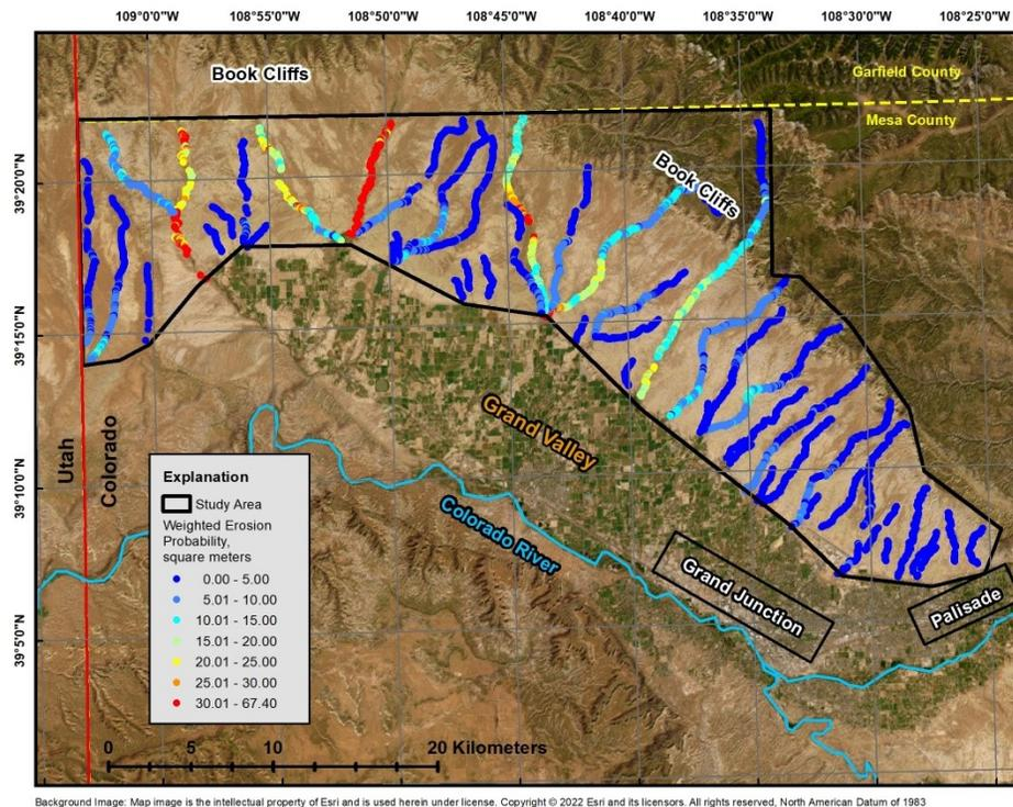
**Figure 3.** Map of cross section streamflow area weighted (multiplied by the cross-sectional streamflow areas) erosion probabilities for the 48 stream channels using 13,415 cross sections in Grand Valley, Colorado (Homan, 2023).
