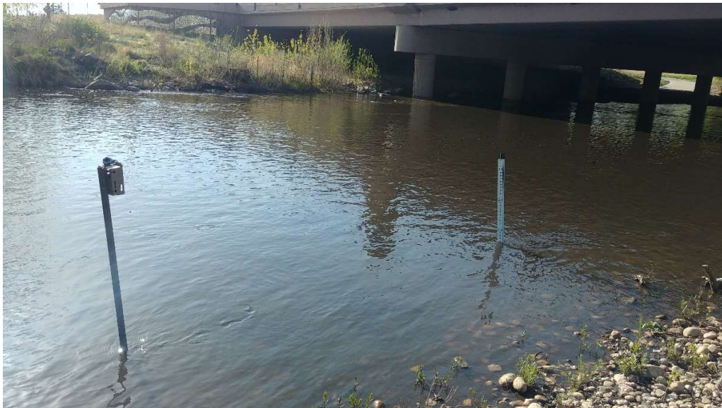
Figure 5. Static stream gage and timelapse camera at the right bank edge of the gravel/cobble bar.
