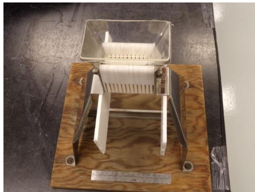
Figure 1. Micro-splitter, 2mm vane spacing. Particles pass through the splitter and drop two inches onto the imaging plate. The white panels below the vanes prevent particles from bouncing away from the designated area.
