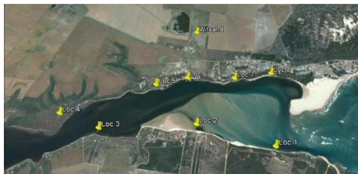
Figure 12. Eight critical locations selected for wave runup calculations in the lower estuary
