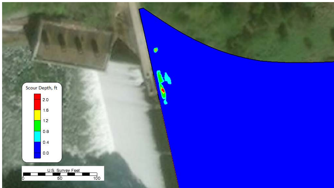
Figure 17. Scour depths near the gate
