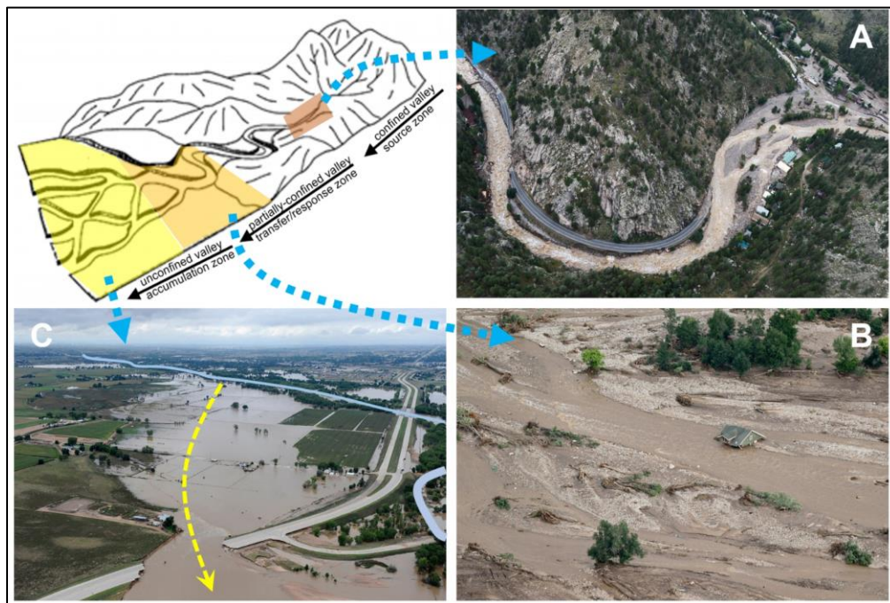
Figure 4. Example of landscape units and dominant flood response within a watershed from mountain headwaters to plains. A) A confined reach in the canyons of the Colorado Front Range Foothills responds to a flood with incision and widening, though braiding and deposition can occur at smaller scales in floodplain pockets. B) A partially confined reach at the transition from canyons to plains responds with lateral migration and braiding. C) an unconfined reach in the plains responds with bank erosion and avulsion. Here the light blue line designates the main channel and the yellow dashed line the avulsion pathway. Adapted from Brierley and Fryirs (2005).
