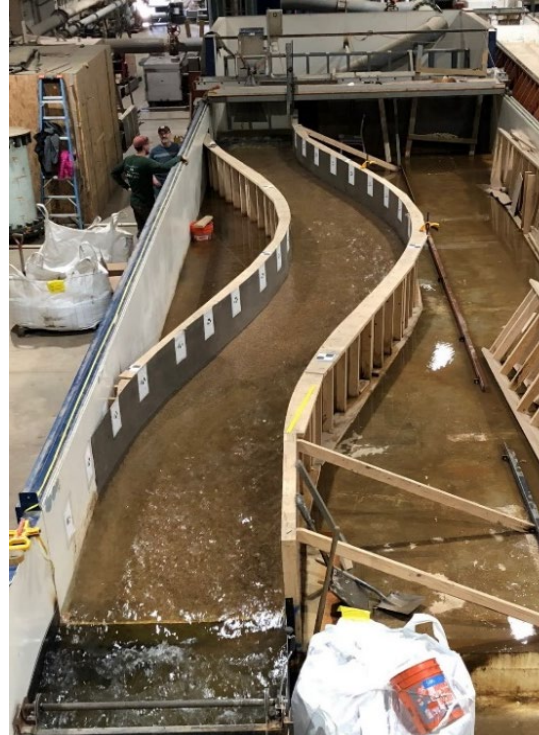
Figure 1. The channel where both experiments were conducted. Flow is from the top of the photo to the bottom. Sediment feeder is visible on scaffolding at upstream end.
