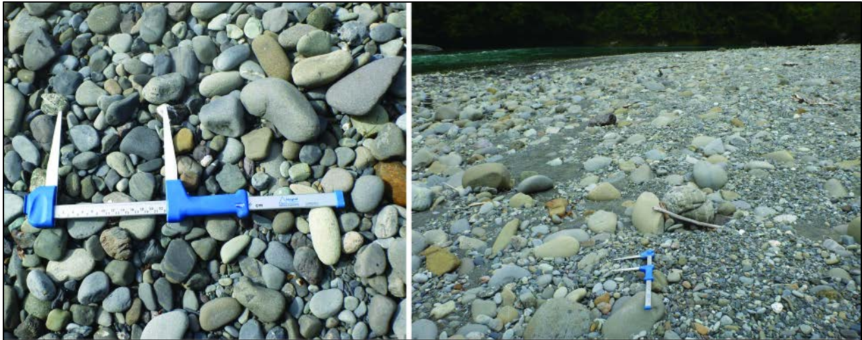
Figure 7. Photographs of Elwha River bed material. Dimensions of 200 bed particles were measured with calipers on three axes.
