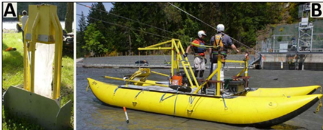
Figure 4. A – TR-2 used for bed load measurements. B – Cataraft used for bed load measurements. The TR-2 is mounted on the downstream side of the raft, operated with a crane and winch.
