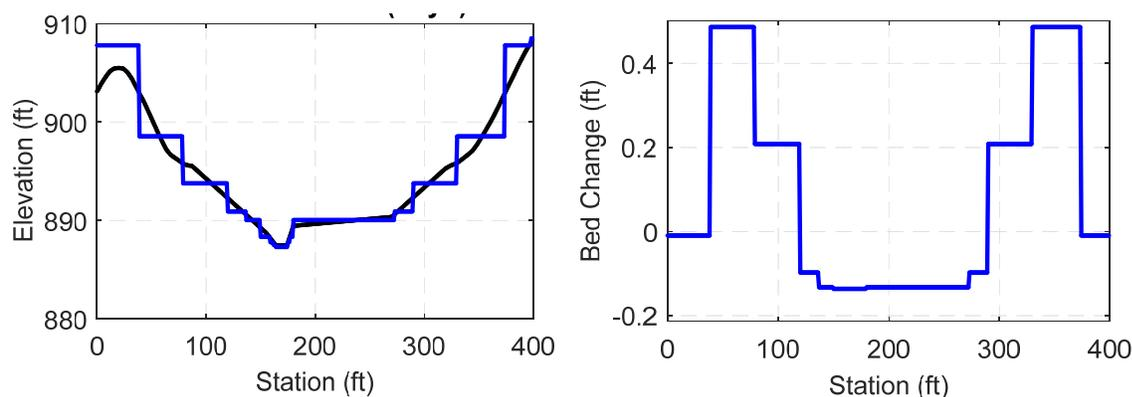
**Figure 5.** Example subface bed elevations and bed change after approximately 12.8 years of simulation for the West Fargo Diversion Canal, North Dakota.
