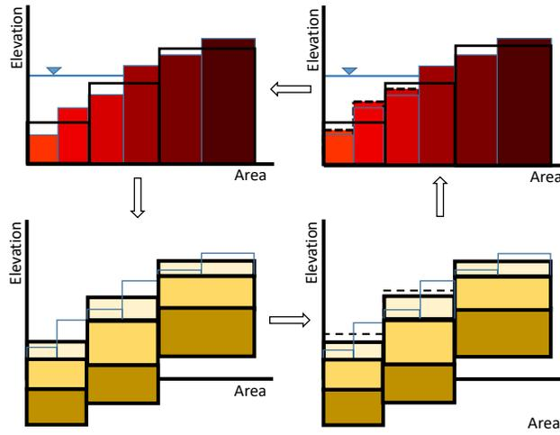
**Figure 2.** Schematic representing computation of bed change.
