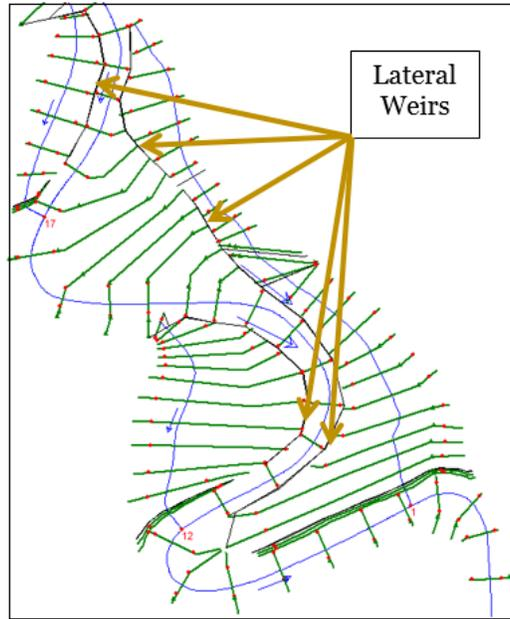
Figure 2. Model geometry approach to floodplain flow.
