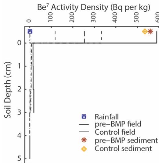
**Figure 5.** Preliminary  $^7\text{Be}$  results from the Indiana edge-of-field sites for the 3/30/2018 event. Pre-event cores indicate  $^7\text{Be}$  is only in the organic-litter layer and very near the surface in the soil profiles in these fields, with no  $^7\text{Be}$  measurable below 5 cm. Differences among individual cores could be due to particle size and organic matter content differences as well as gamma counting differences for low-mass organic samples on the top of the profiles.
