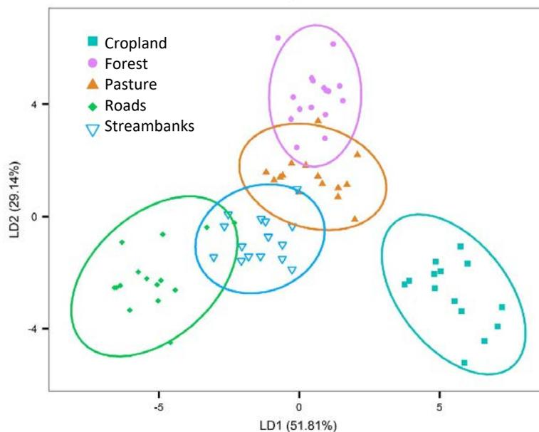
**Figure 2.** Preliminary source discrimination for September-October sediment from Black Creek gage site. LD1 is the indicator that provides the most differentiation (51.81%) among the sources - this is Zirconium. LD2 is the next most differentiating indicator - Tungsten. Eight critical indicators were identified.
