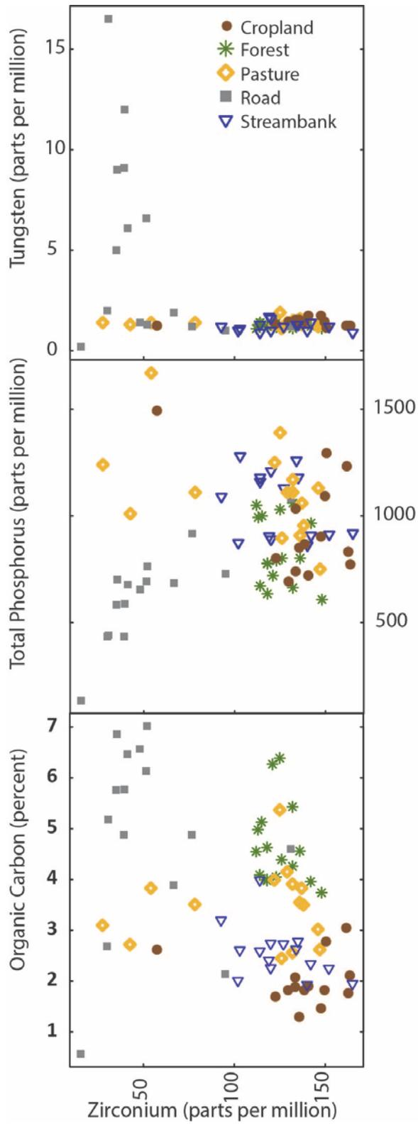
**Figure 3.** Concentrations of indicators. Preliminary analysis identified zirconium and tungsten as the two indicators that best separate the sources. Organic carbon and total phosphorus in sediment significantly improve this differentiation; their relative abundance reflects what we would expect from these five environments.
