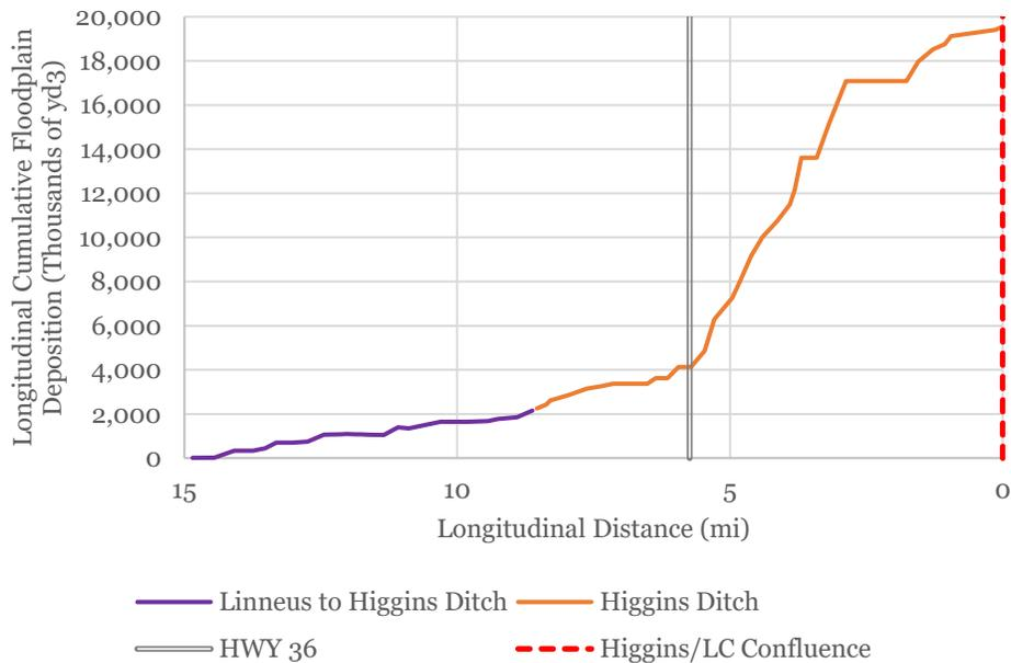
**Figure 3.** Longitudinal Cumulative Volume Curve
