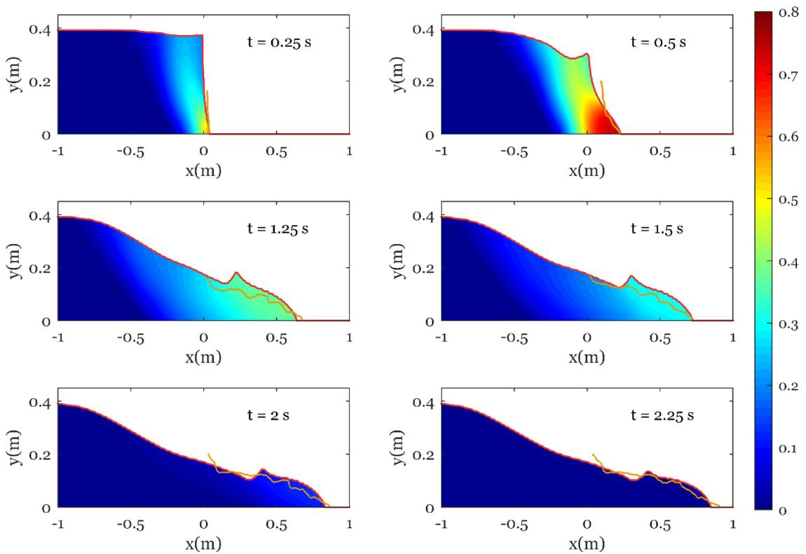
**Figure 5.** Comparison of the mixture profiles between the simulation (red line) and the experiment (yellow line), and velocity magnitude for the simulation at different times.
