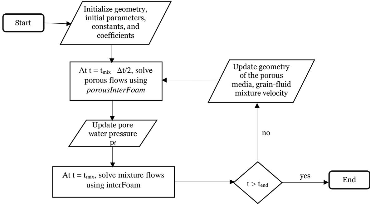
**Figure 1.** Detailed relationship of *porousMixtureInterFoam* algorithm.
