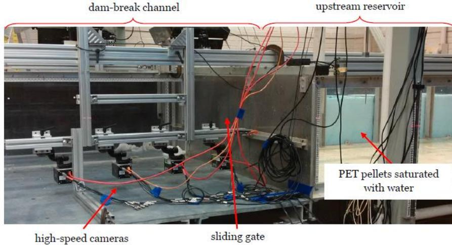
**Figure 3.** Experimental setup (Rebillout et al., 2017).
