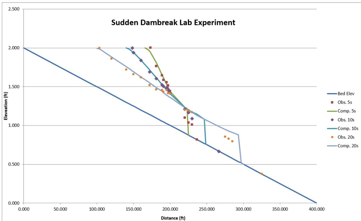
**Figure 3.** Original Shallow Water Solver vs Lab Results.
