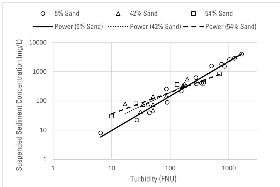
**Figure 3.** Regression lines for Turbidity-SSC models based on grain size
