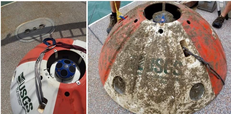
**Figure 2.** USGS barnacle before deployment and immediately after recovery with hydroacoustic instrumentation used for the study.
