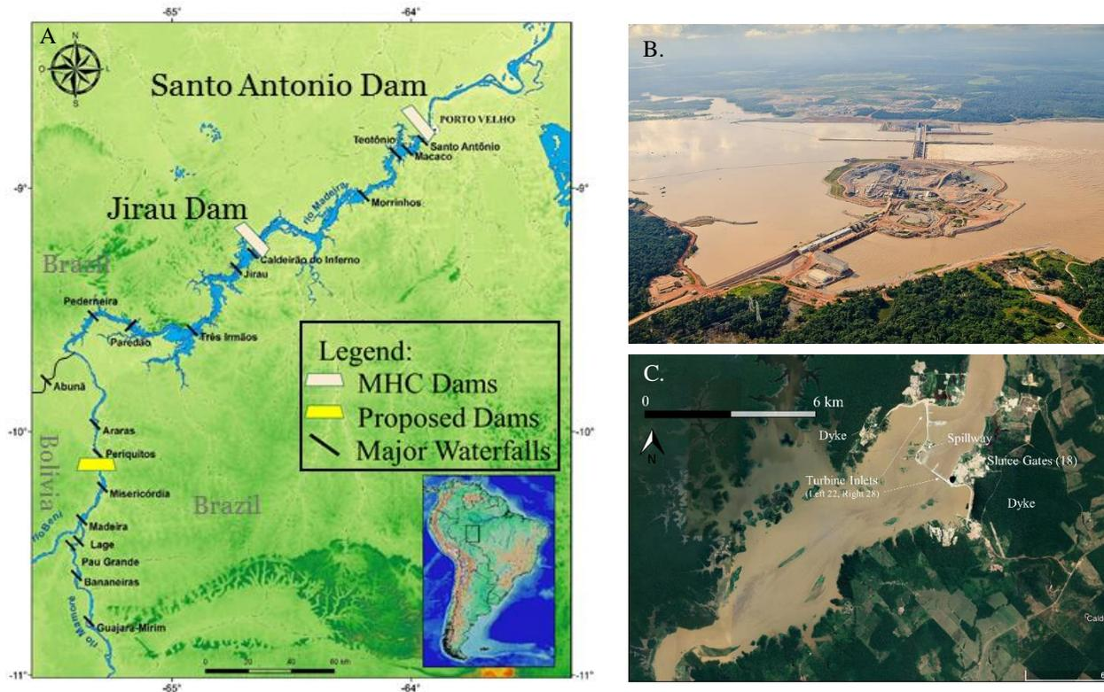
**Figure 1.** A. Santo Antonio and Jirau dam locations along the Madeira River in Rondonia, Brazil (Modified from Cella-Ribeiro et al 2013); B. Santo Antonio Dam under construction (skyscrapercity.com); C. Jirau Dam with major components and scale for reference (Google Earth).
