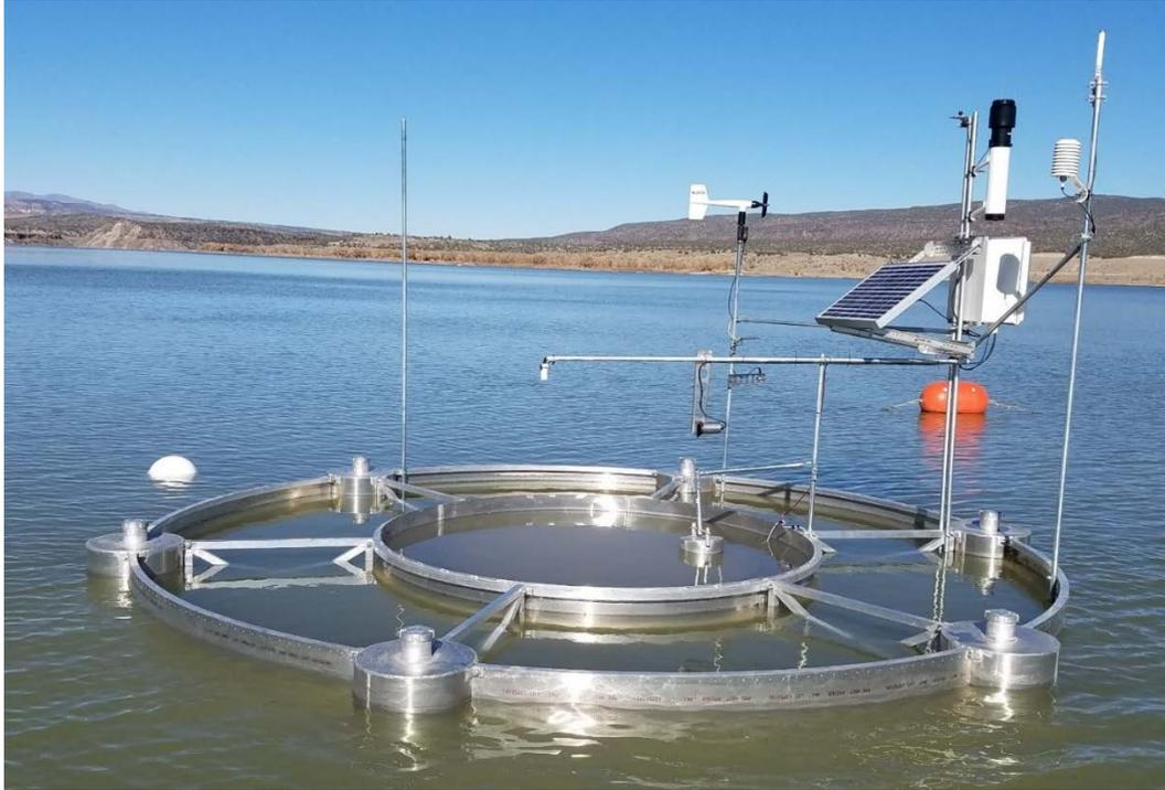
**Figure 1.** Collision Floating Evaporation Pan (CFEP) on Cochiti Lake, New Mexico (8-foot diameter evaporation pan and 16-foot diameter outer wave guard).
