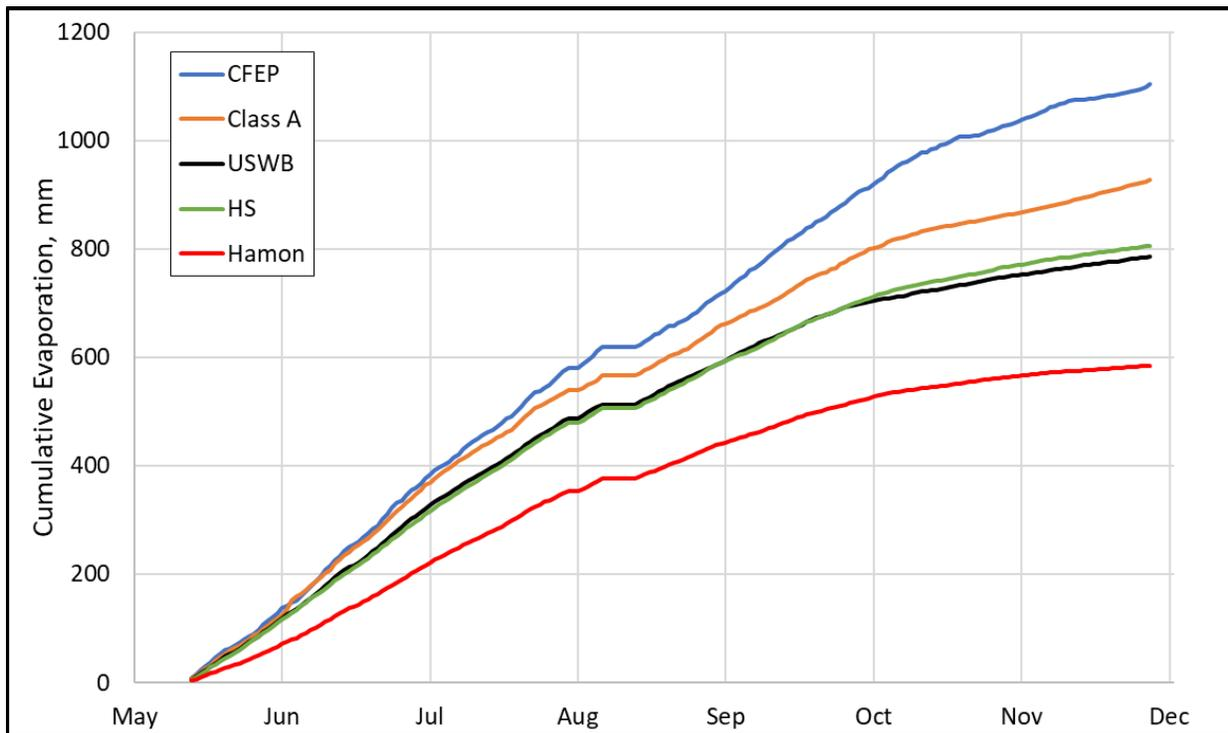
**Figure 2:** Cumulative evaporation for the CFEP (Collision Floating Evaporation Pan), Class A Pan, USWB equation (U.S. Weather Bureau), HS equation (Hargreaves-Samani), and Hamon equation.
