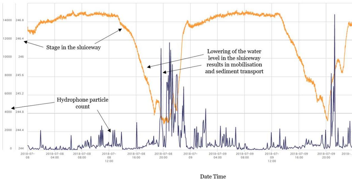
**Figure 5. Sluiceway stage and hydrophone particle count between July 8<sup>th</sup> and 10<sup>th</sup>, 2018.**
