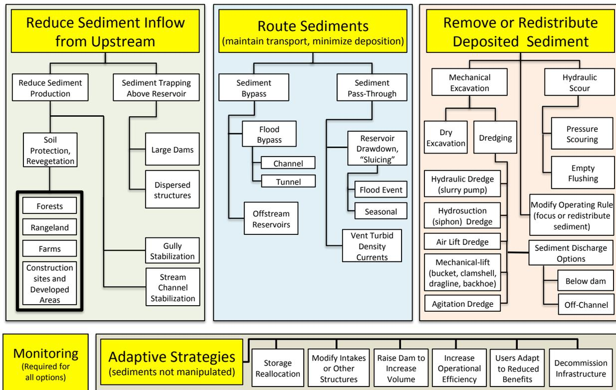
Figure 6: Methods for managing reservoir sedimentation (after Morris 2015).
