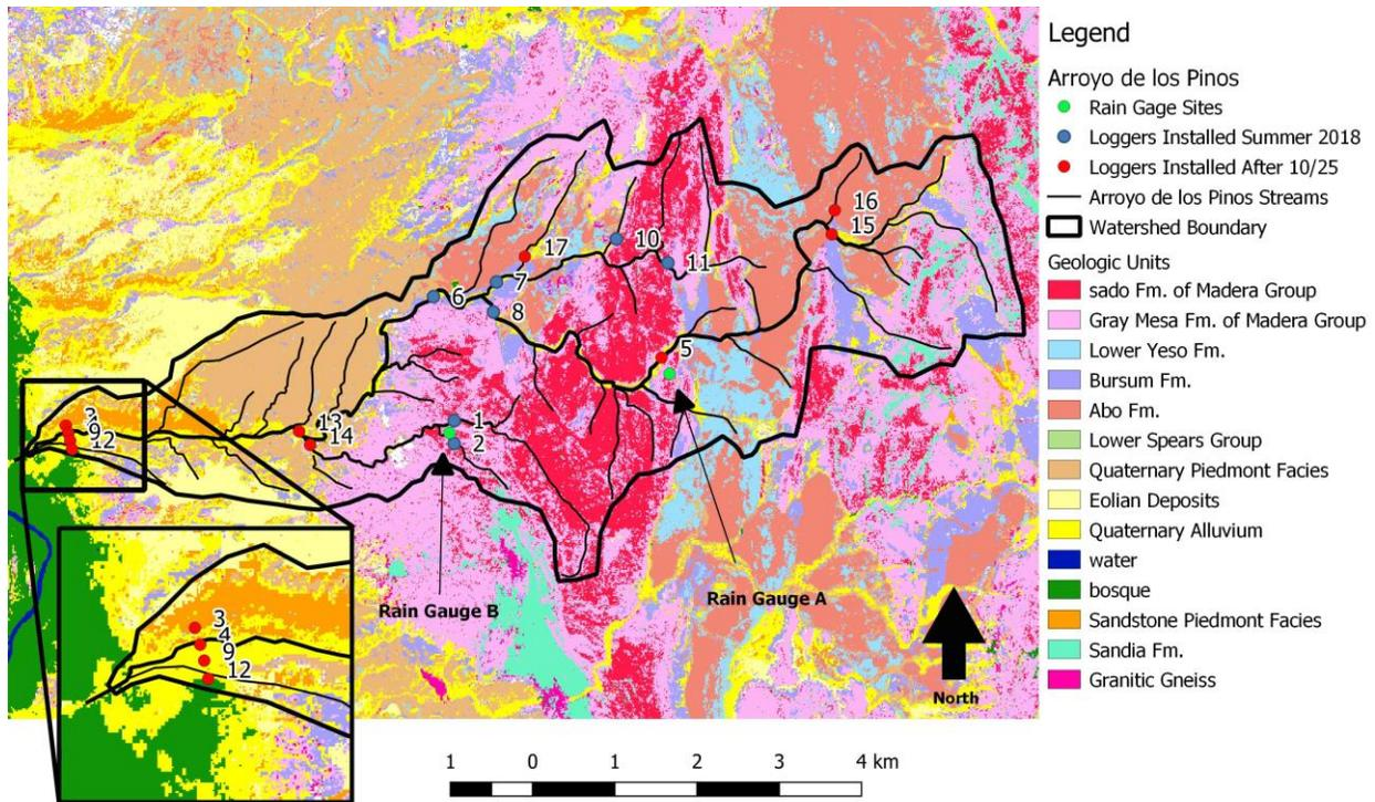
**Figure 1:** Arroyo de los Piños pressure transducer and rain gauge sites, with inset of closely placed pressure transducers in the lower braided reach. The underlying geologic map is adapted from Cather 2005. Red circles are pressure transducers installed after the two storms looked at in this paper (we do not have flood data at these sites).
