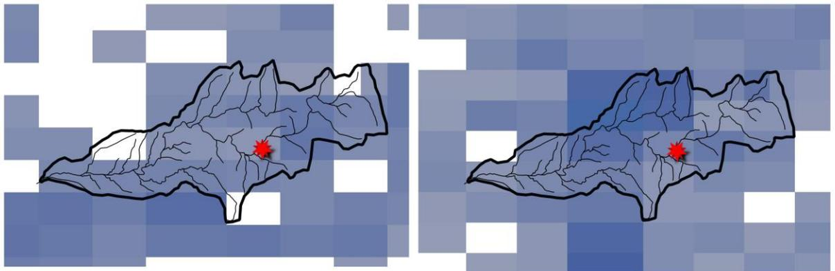
**Figure 6:** NEXRAD reflectivity raster for October 2<sup>nd</sup> storm. The left image is from 17:00, and the right is from 18:00. The red star shows the location of the rain gauge used in this analysis.
