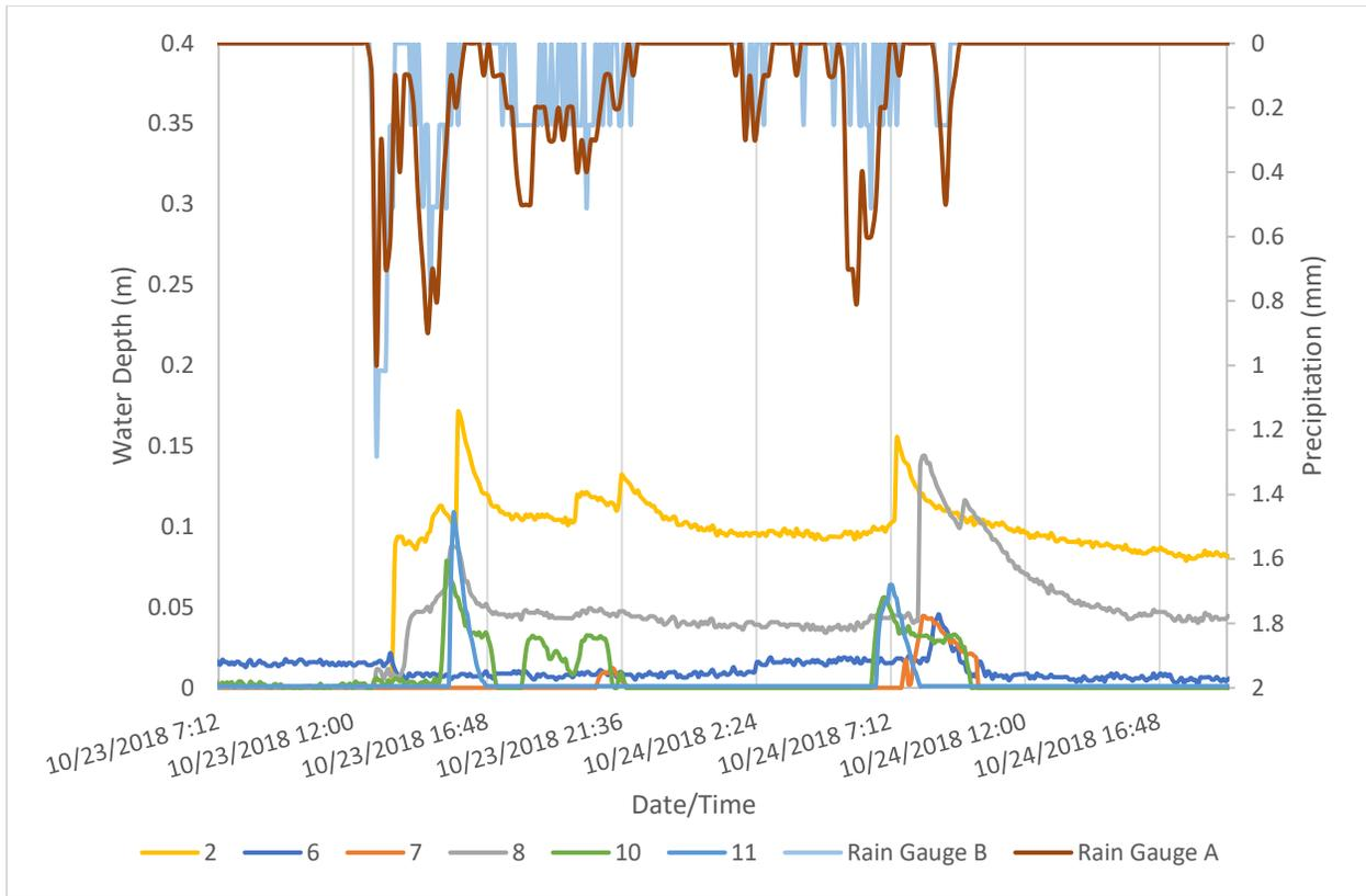
**Figure 3:** Tributary histograms for October 23. Flow was initiated at pressure transducer 2 in the southern portion of the basin, quickly followed by flow at 8, 10, 11, and 7 in the northern part of the basin.
