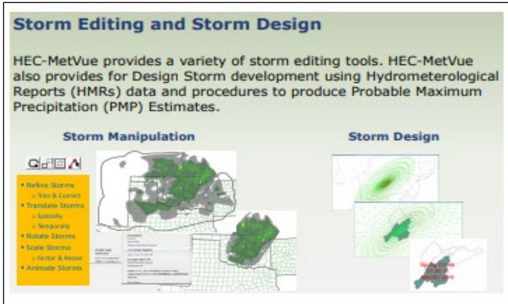
**Figure 3.** Storm Editing and Storm Design in HEC-MetVue
