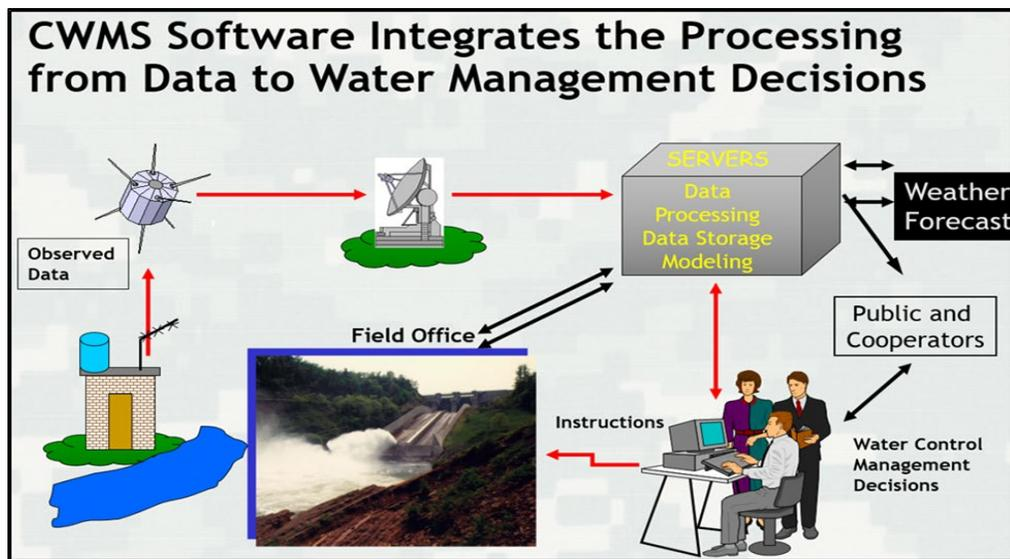
Figure 1. Picture of CWMS an Automated Information System
