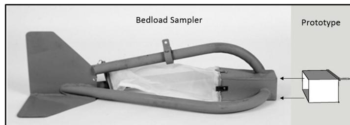
**Figure 2.** BL-84 bedload sampler and prototype of proposed attachment
