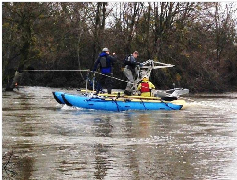
**Figure 1.** Tetra Tech engineers sampling bedload on the San Joaquin River in January 2017
